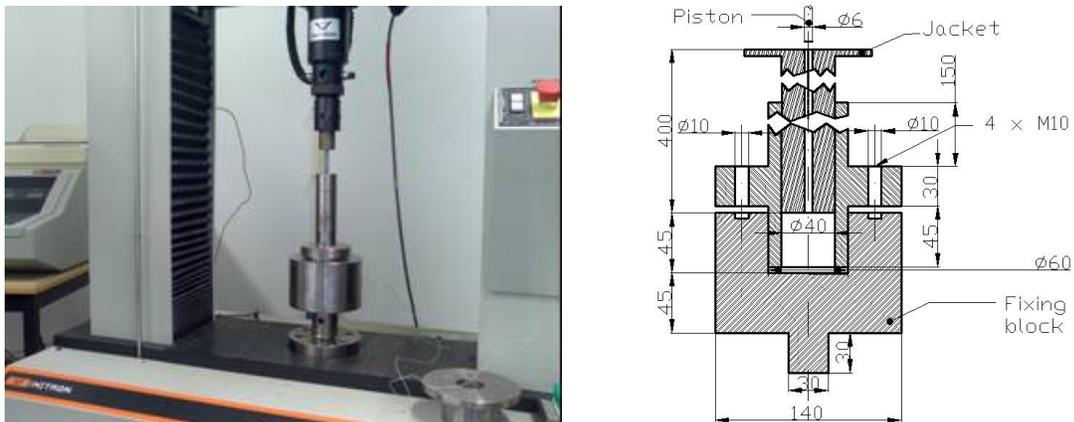
Figure 3. Instron machine and drawing sectional view of the pellet compression chamber.
