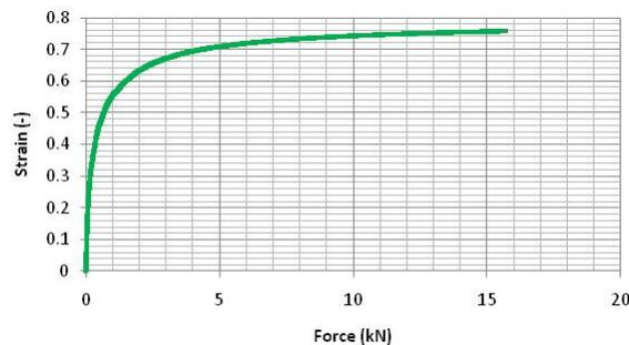
Figure 5. Strain change with load during a 10 mm diameter pellet test manufacture.
