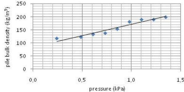
Figure 3. Pile bulk density versus applied pressure.
