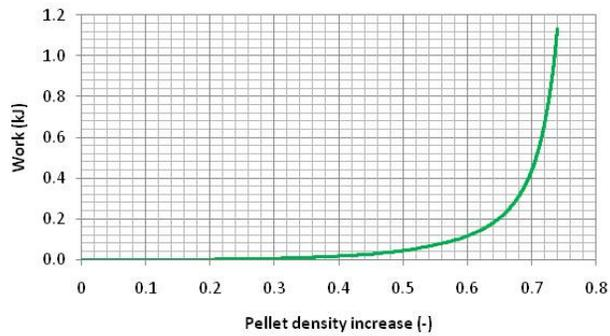
Figure 7. Diagram of the energy spent versus densification of a 10 mm diameter pellet to 74% using a load rate of 1.0 MPa/s (4710 N/min for a 10 mm diameter).
