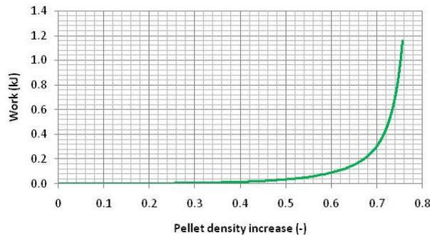
Figure 6. Diagram of the energy spent versus densification of a 10 mm diameter pellet to 76% .
