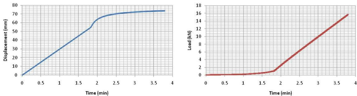
Figure 4. Displacement and load change with time during a 10 mm diameter pellet test manufacture.
