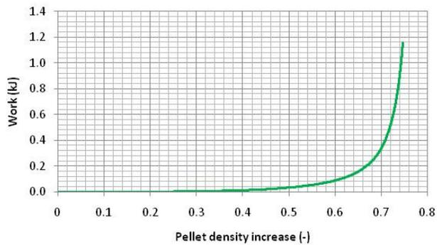
Figure 8. Diagram of the energy spent versus densification of a 10 mm diameter pellet to 75% using a load rate of 0,5 MPa/s (2365 N/min for a 10 mm diameter).
