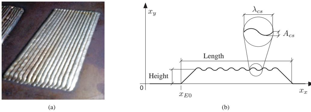
Figure 4. Strips of solder profile: (a) real and (b) approximated.
