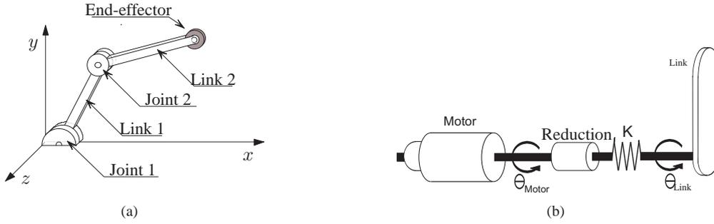
Figure 1. (a) Service manipulator and (b) joint model
