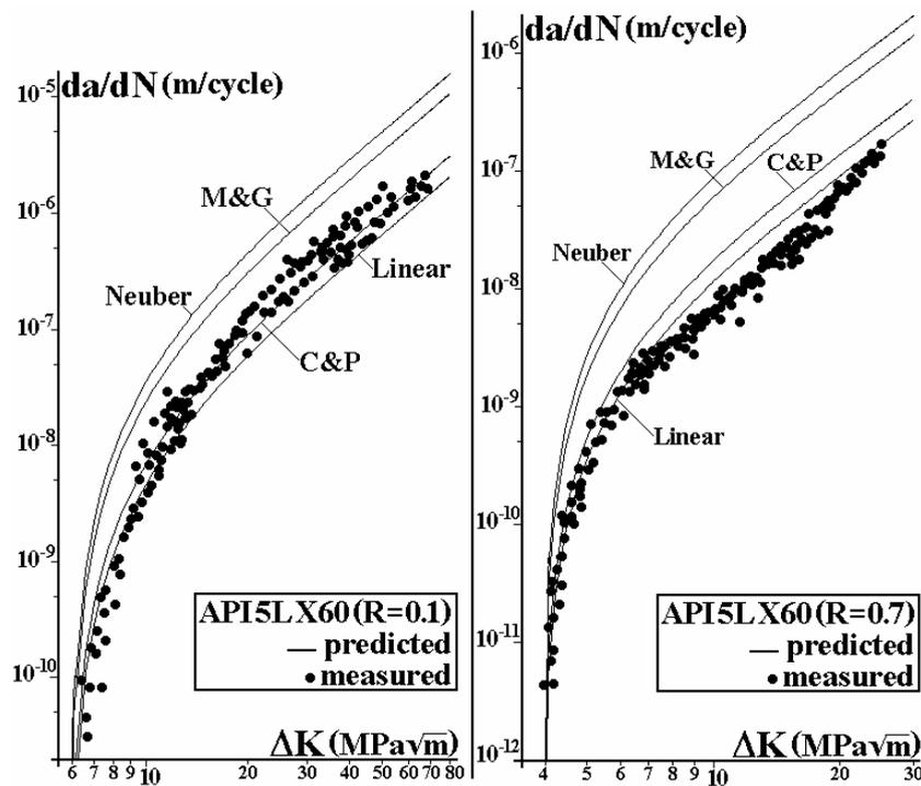
Fig. 2.  $da/dN \times \Delta K$  behavior measured and predicted by the various strain concentration rules used in the critical damage model, for API-5L-X60 pipeline steel at  $R = 0.1$  and  $R = 0.7$ .
