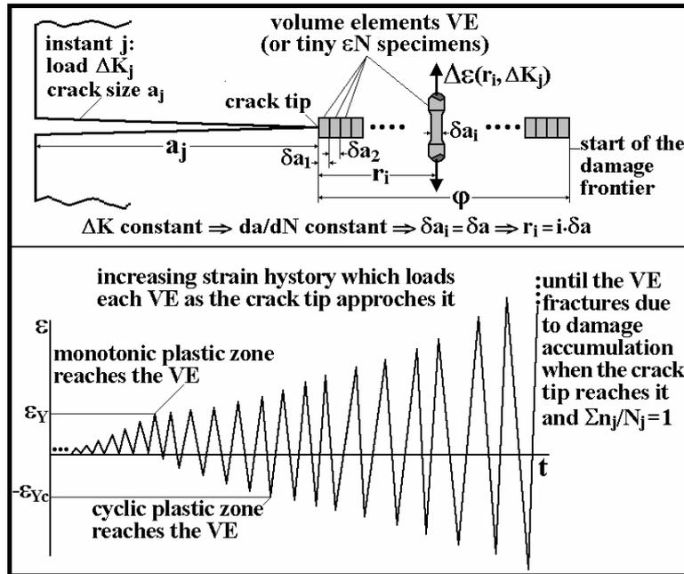
Fig. 1. Schematics of the FCG assumed to be caused by the sequential fracture of volume elements (or tiny  $\epsilon N$  specimens) at every load cycle, loaded by an increasing strain history as the crack tip approaches them.
