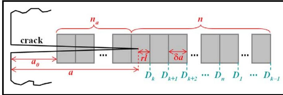
Fig. 6. Volume elements before and ahead of the crack tip, showing the main length parameters and the locations for the calculation of the accumulated damages  $D_1$  through  $D_n$ .
