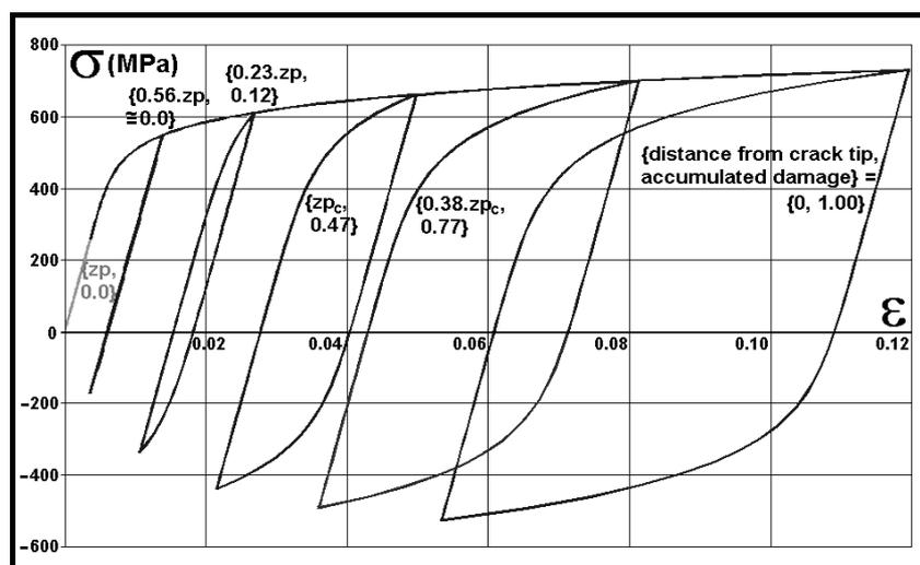
Fig. 5. Schematics of the loops at a fixed VE at different crack growth stages, under constant  $\Delta K$  loading, showing that an accumulated damage of 0.47 is already present in this VE when it is reached by the cyclic plastic zone  $z_{p_c}$ .
