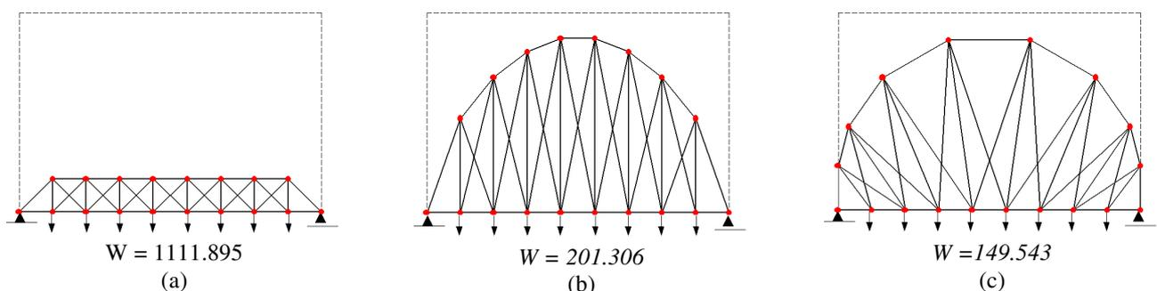
Figure 3. (a) Initial structure ( $L_x = 9$ ,  $L_y = 1$ ,  $D_x = 9$ ,  $D_y = 6$ ). Optimum geometry considering as design variables (b) the  $y$  coordinates only, and (c) both  $x$  and  $y$  coordinates of the upper chord nodes.
