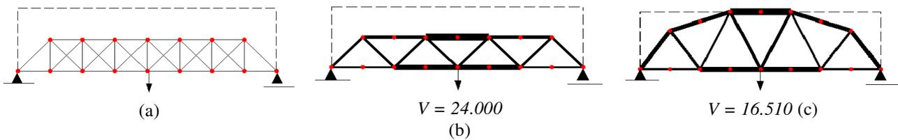
Figure 5. (a) Initial structure ( $L_x = 8, L_y = 1, D_x = 8, D_y = 2$ ). (b) Optimum topology. (c) Optimum design from simultaneous geometry and topology optimization, considering the  $y$  coordinates of the upper chord nodes as design variables.
