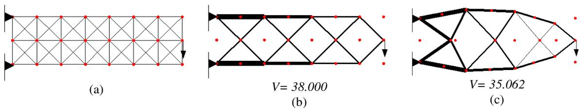
Figure 6. (a) Initial structure ( $L_x = 7, L_y = 2$ ). (b) Optimum topology. (c) Optimum design from simultaneous geometry and topology optimization, considering as design variables the  $x$  and  $y$  coordinates of the upper and lower chord nodes, and the  $x$  coordinates of the nodes aligned with the applied load. Bounds on the design variables are defined locally, by a square of size  $b = 0.8$  centered at the original node position.
