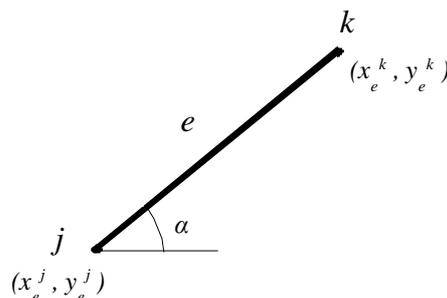
Figure 1. Cartesian coordinates  $x$  and  $y$ , initial node  $j$ , end node  $k$ , and inclination angle  $\alpha$ , measured in the anti-clockwise direction, for the element  $e$ .
