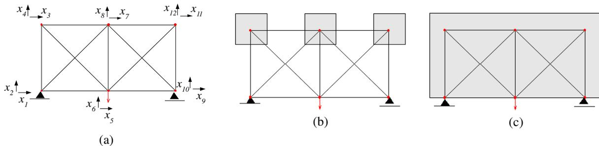
Figure 2. (a) Truss structure with nodal coordinates as design variables. The gray rectangles in (b) and (c) represent the feasible domains, bounded by box constraints on the nodal coordinates: bounds can be defined (b) locally for each design variable separately, and (c) globally for all the design variables at once.
