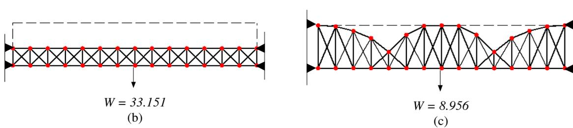
Figure 4. (a) Initial structure ( $L_x = 14, L_y = 1, D_x = 14, D_y = 2.5$ ). (b) Optimum geometry considering the  $y$  coordinates of the upper chord nodes as design variables.
