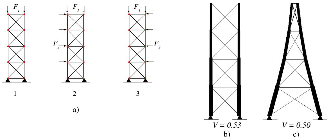
Figure 7. a) Initial structure subjected to three alternative loading conditions ( $L_x = 1, L_y = 4$ ), considering  $F_1 = 10$  and  $F_2 = 1$ . Results from b) only topology optimization and c) simultaneous optimization of geometry and topology. In the geometry optimization step all nodes are allowed to “move” left and right. Bounds on the design variables for the geometry optimization are defined locally, by a square of size  $b = 0.4$  centered at the original node position.
