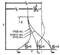
Figure 7. Boundary-layer temperature distribution.
