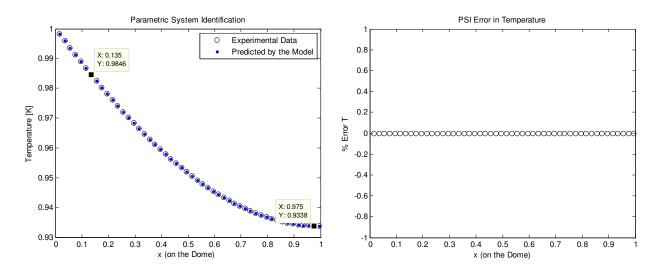
Figure 10. PSI method with Radiation term.
