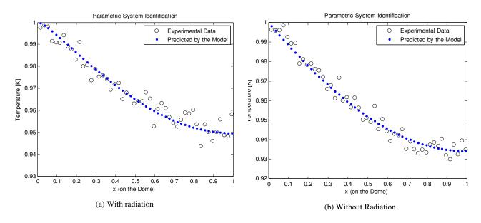
Figure 11. PSI method with noise and radiation (20 seconds).
