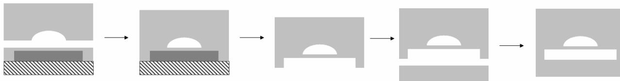
Figure 5. Multilayer PDMS bonding sequence via oxygen plasma treatment.
