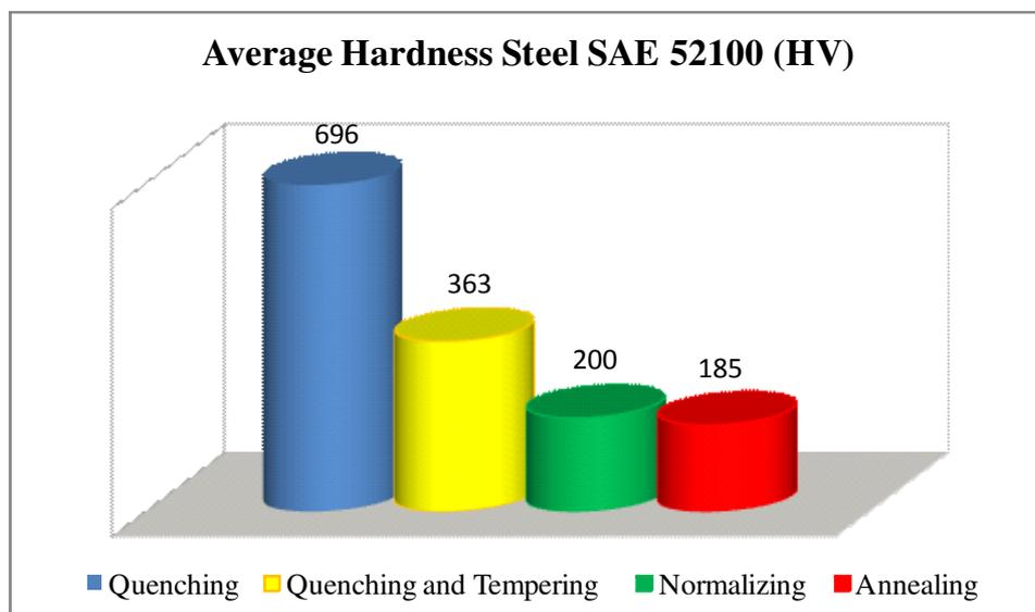
Figure 3 - Hardness of the specimens in scale HV.
