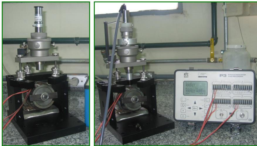
Figure 2 – Complete equipment for residual stresses measurements with the bearing cone parts.
