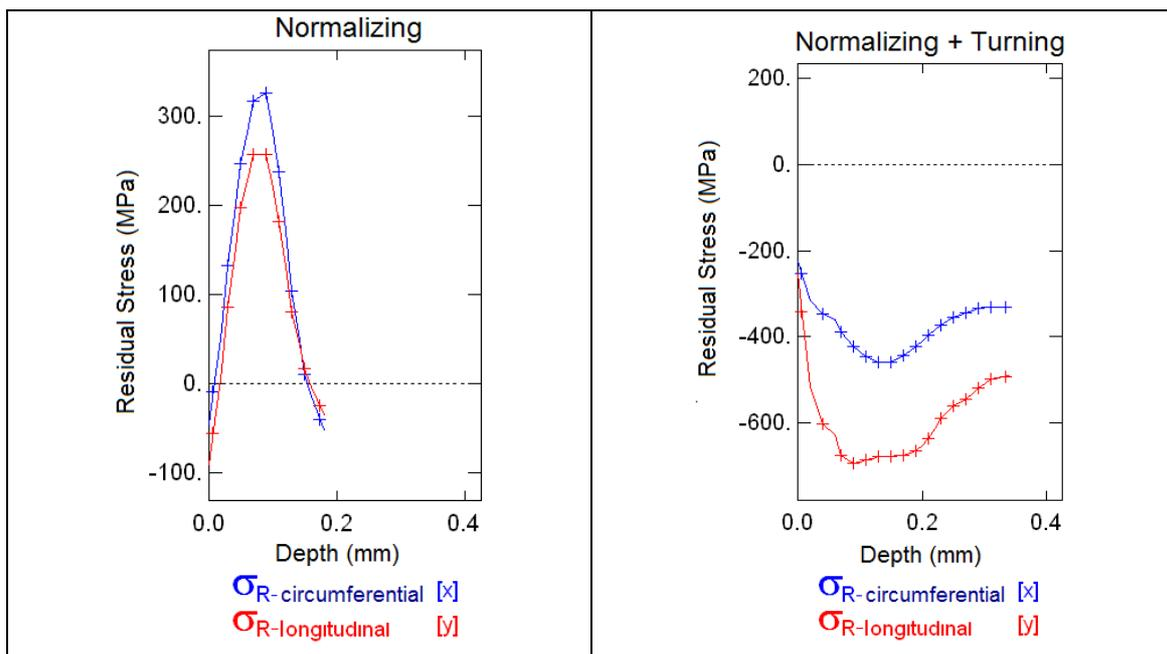
Figure 6. Residual stress measurements for the normalized piece
