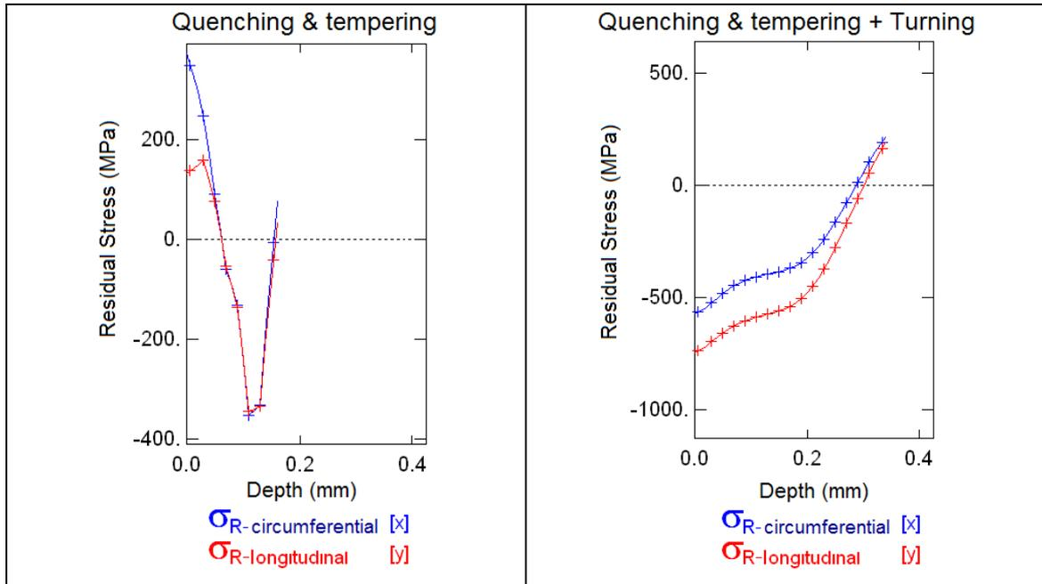
Figure 7. Residual stress measurements for the quenched and tempered piece
