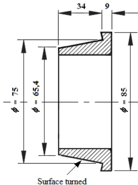
Figure 1 - Conical bearing part used in the tests
