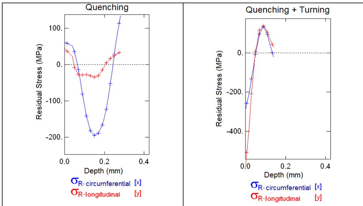
Figure 8. Residual stress measurements for the quenched piece
