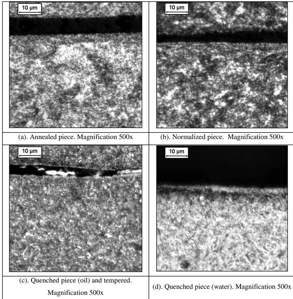
Figure 4. Microstructure of different heat treatments and turning.
