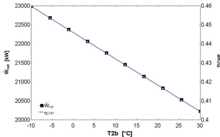
Figure 4. Effect of the inlet air temperature in power generation and efficiency - case 2.
