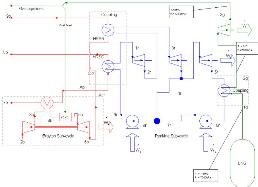
Figure 2. CHP cycle coupled to a LNG re-gasification plant – case 1.
