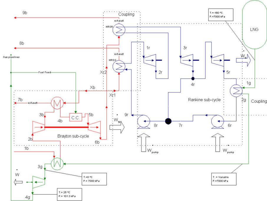
Figure 3. CHP cycle coupled to a LNG re-gasification plant – case 2.
