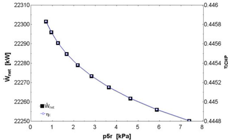
Figure 5. Effect of the outlet pressure of Rankine sub-cycle low pressure turbine on the energy production and efficiency - case 2.
