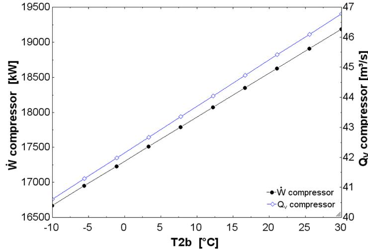
Figure 6. Effect of Brayton sub-cycle inlet air temperature on the compressor volumetric flow rate and power consumption.
