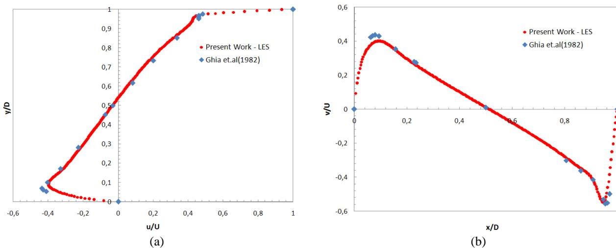
Figure 3. Dimensionless velocity profiles for  $Re = 5000$ .
