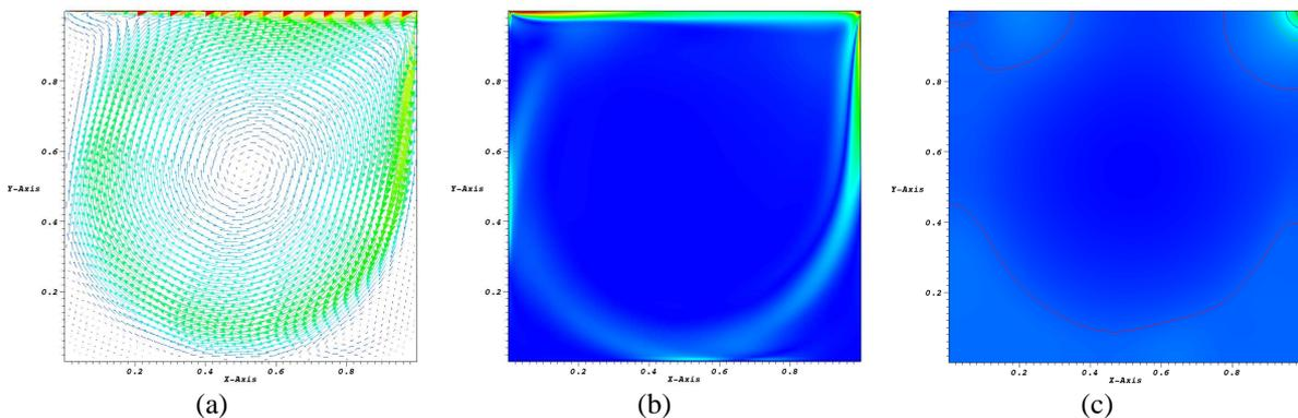
Figure 6. Maps of (a) velocity vector, (b) eddy viscosity and (c) pressure field for  $Re = 3200$ .
