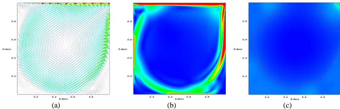
Figure 9. Maps of (a) velocity vector, (b) eddy viscosity and (c) pressure field for  $Re = 10000$ .
