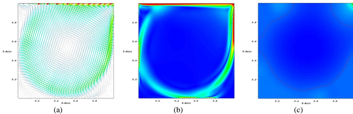
Figure 8. Maps of (a) velocity vector, (b) eddy viscosity and (c) pressure field for  $Re = 7500$ .
