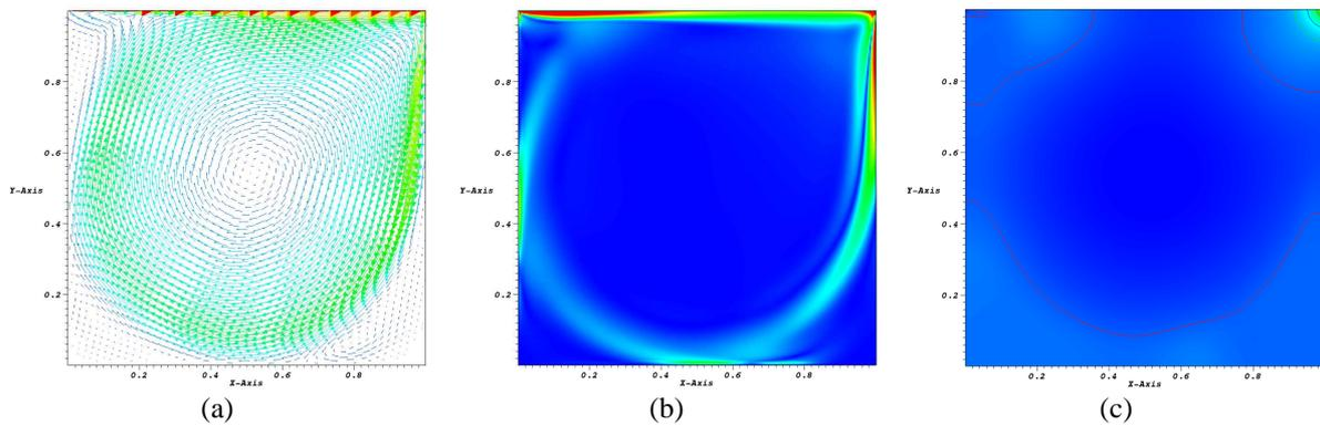
Figure 7. Maps of (a) velocity vector, (b) eddy viscosity and (c) pressure field for  $Re = 5000$ .
