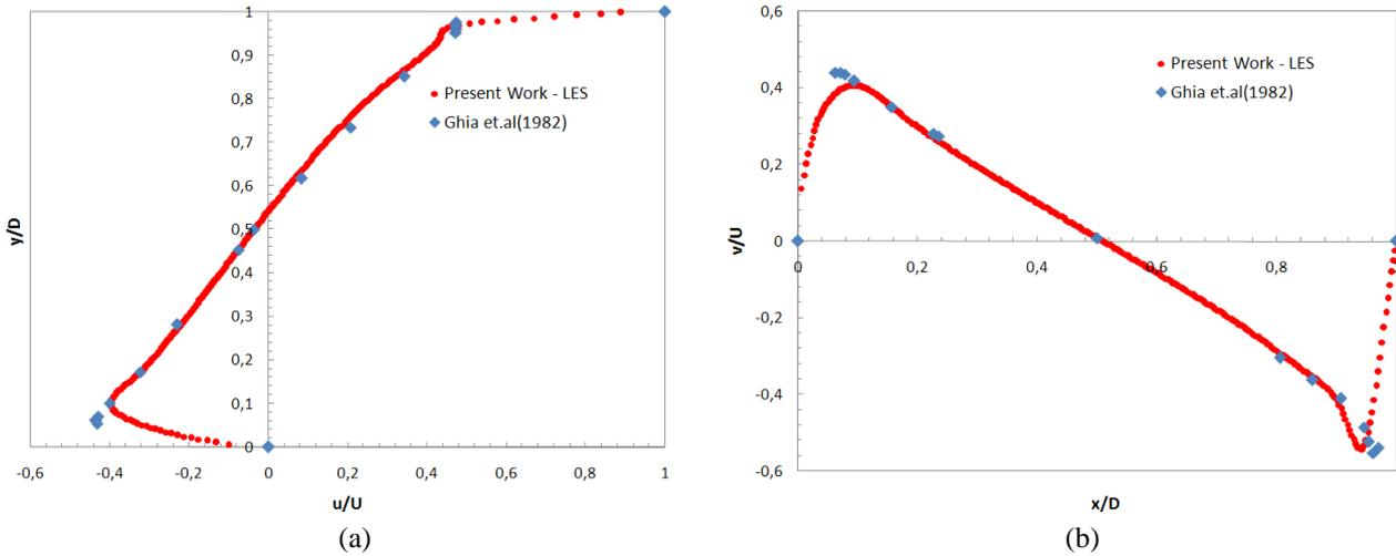
Figure 4. Dimensionless velocity profiles for  $Re = 7500$ .
