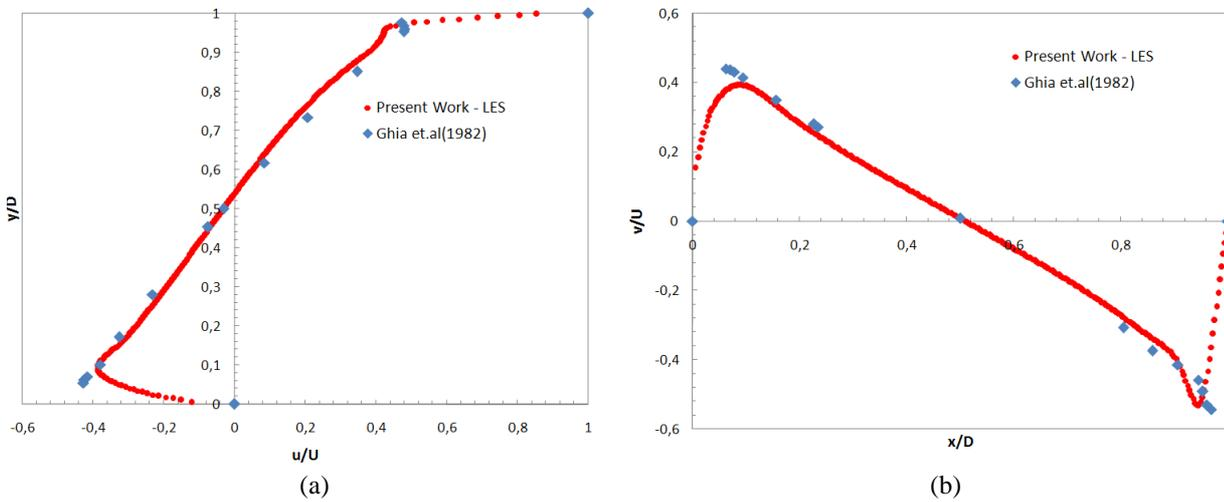
Figure 5. Dimensionless velocity profiles for  $Re = 10000$ .
