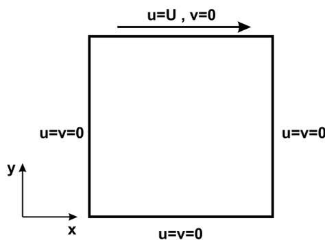
Figure 1. Scheme of the lid-driven square cavity and boundary conditions.
