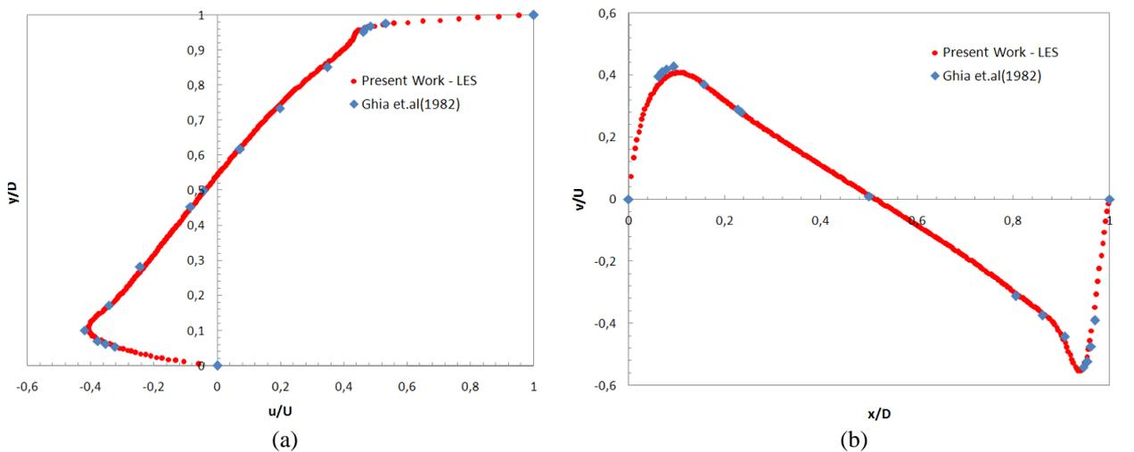
Figure 2. Dimensionless velocity profiles for  $Re = 3200$ .
