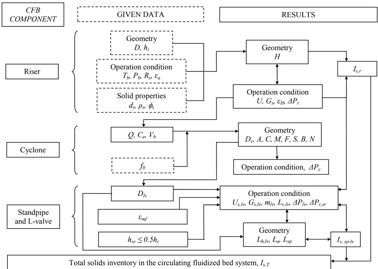
Figure 2. Structure of the semi-empirical model ( $T_b$  and  $P_b$  are the temperature and pressure of the system, respectively).
