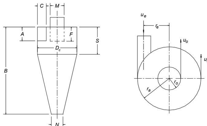
Figure 1. Geometrical configuration of the cyclone.
