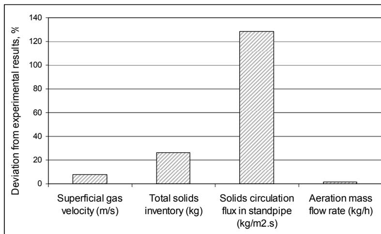
Figure 3. Validation of the semi-empirical model for the main CFB operational variables. Comparison from Hory, *et al*. (2006).
