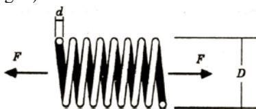
Figure 2. Helical spring.
