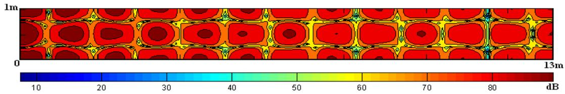
Figure 3a – Sound pressure level inside the simple duct at 400Hz (CMS technique).
