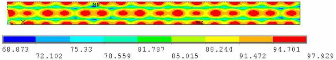
Figure 3b – Sound pressure level inside the simple duct at 400Hz (FEM method).
