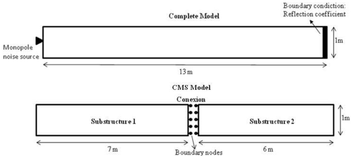
Figure 1 – Duct acoustic of simple geometry
