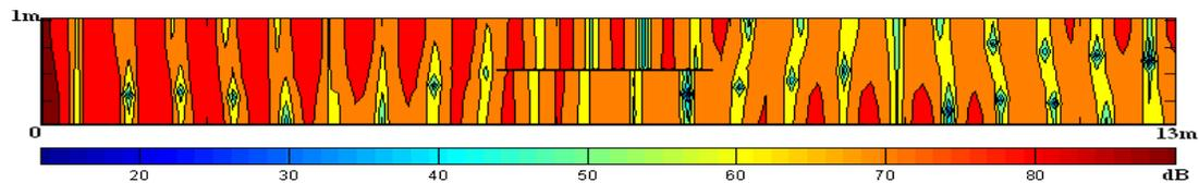
Figure 5a – Sound pressure level inside the duct with a plate at 300 Hz (CMS technique).
