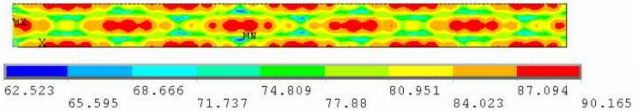
Figure 4b – Sound pressure level inside the simple duct at 500Hz (FEM method).
