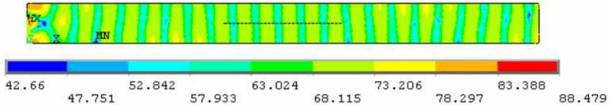
Figure 5b – Sound pressure level inside the duct with a plate at 300 Hz (FEM method).
