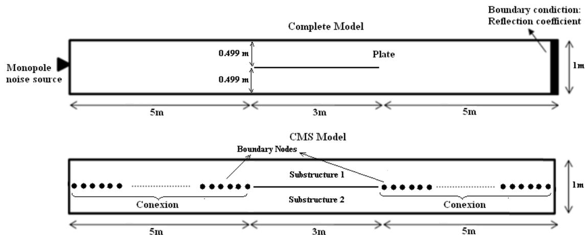
Figure 2 –Duct with a thinner plate inside it.
