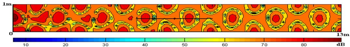
Figure 6a – Sound pressure level inside the duct with a plate at 400 Hz (CMS technique).
