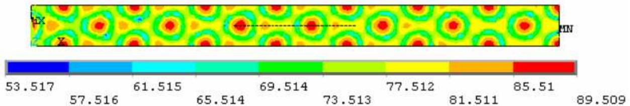
Figure 6b – Sound pressure level inside the duct with a plate at 400 Hz (FEM method).
