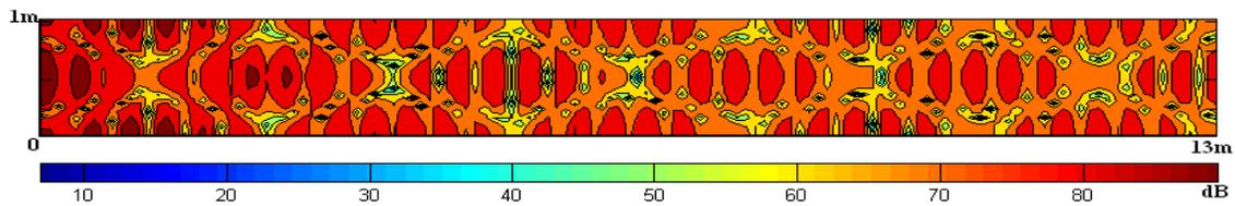
Figure 4a – Sound pressure level inside the simple duct at 500Hz (CMS technique).
