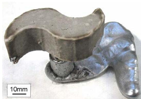
Figure 13. Casting after pouring and solidify.
