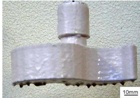
Figure 8. EPS pattern covered with the refractory slurry.
