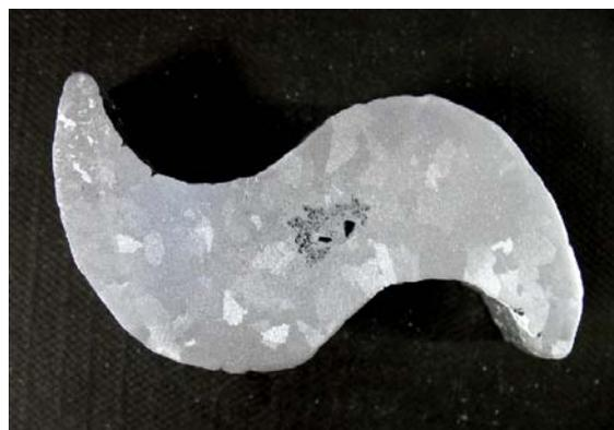
Figure 16. Casting crystalline structure obtained by the lost foam process.
