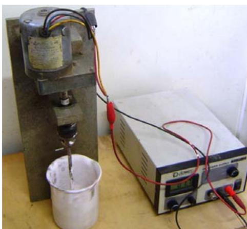
Figure 6. Mounted system to maintain the agitated slurry mixture.
