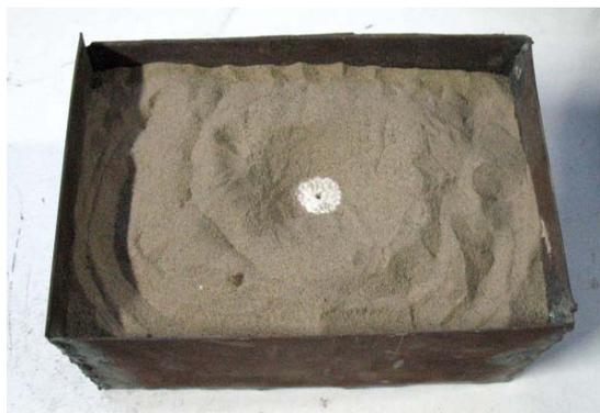
Figure 7. Mold ready to be poured.
