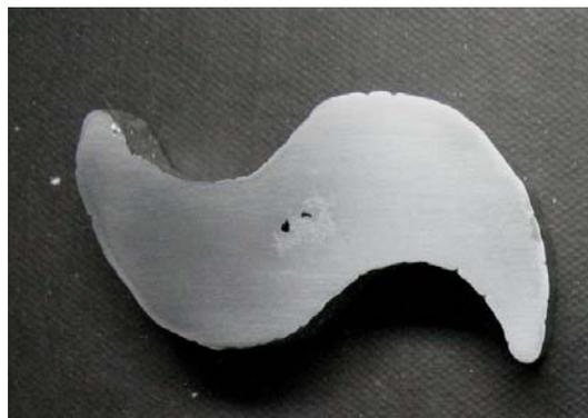
Figure 15. Sanded casting showing the absence of pores of great dimensions.
