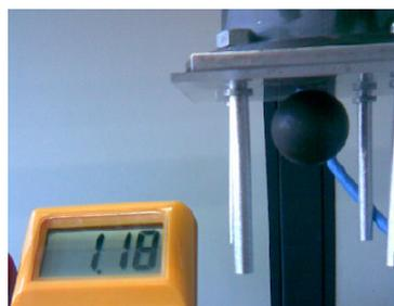
Figure 4. Experimentation to determine the current and the tension values in the equilibrium position.
