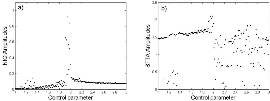
**Figure 4** Resonance curve of the amplitudes for  $\gamma=0.9$  and  $\mu=100$  on the range  $1 \leq a \leq 2.0$  and  $\gamma=0.01$  and  $\mu=100$  on the range  $2.01 \leq a \leq 3.0$ : a) NIO, b) STTA.
