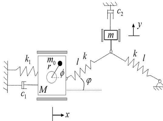
**Figure 1 Schematic of a non-ideal structure attachment coupled to snap-through truss absorber**
