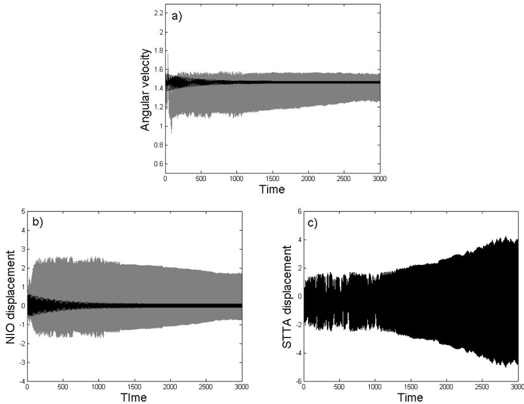
**Figure 6 Time histories for  $a=2.2$ : a) angular velocity, b) NIO response, c) STTA response. STTA off (black diagram) and STTA on (gray diagram).**
