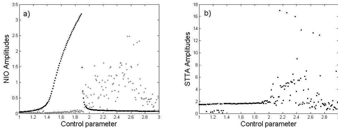
**Figure 3 Resonance curve of the amplitudes: a) NIO without STTA (black points), with STTA (gray points); b) STTA (black points)**
