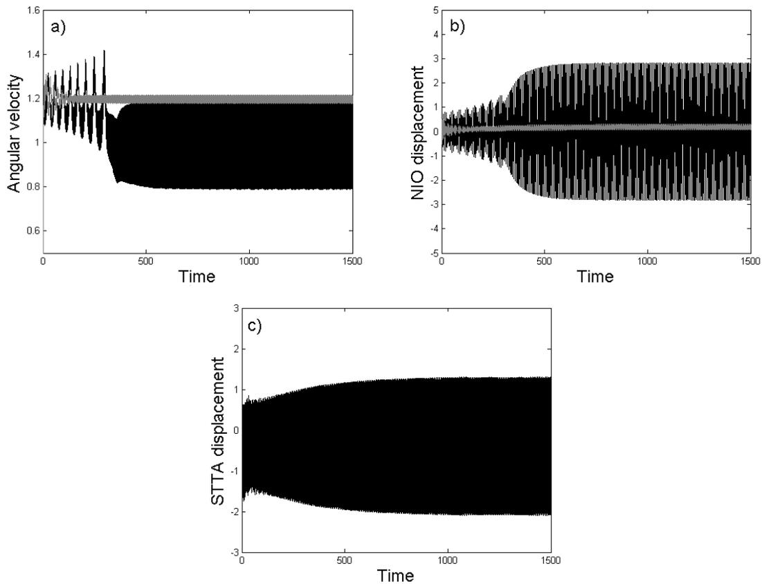
**Figure 5** Time histories for  $a=1.8$ : a) angular velocity, b) NIO response, c) STTA response. STTA off (black diagram) and STTA on (gray black).
