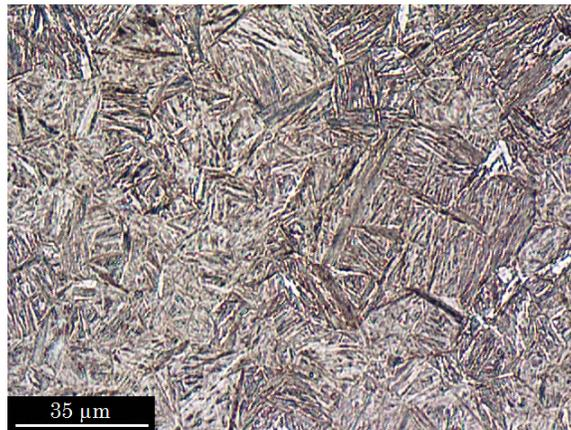
Figure 3. Optical micrograph of water-quenched AISI 1045 sample steel (etched with nital 3%).
