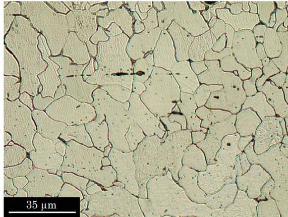
Figure 1. Optical micrograph of an AISI 1006 sample steel (etched with nital 3%).
