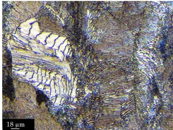
Figure 2. Optical micrograph of an AISI 1080 sample steel (etched with nital 3%).
