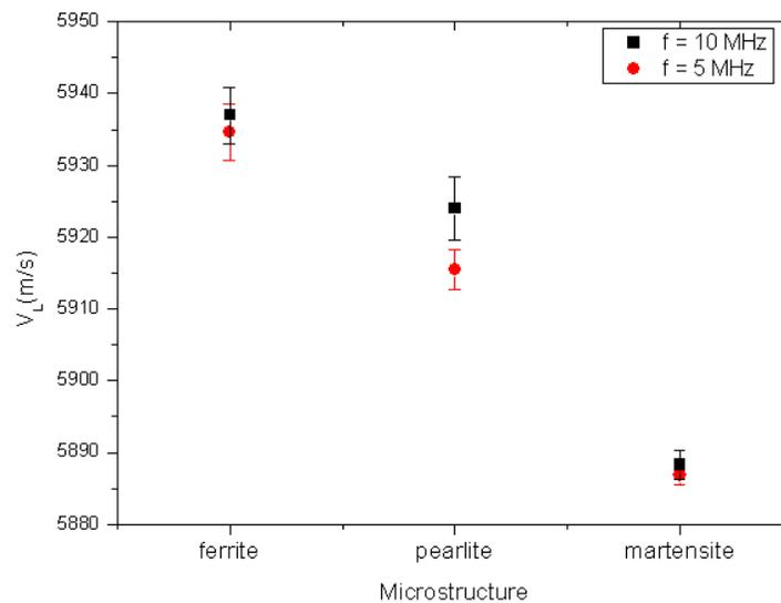
Figure 5. Correlation between microstructures and longitudinal ultrasonic velocities ( $V_L$ ) in frequencies of 5 and 10MHz.
