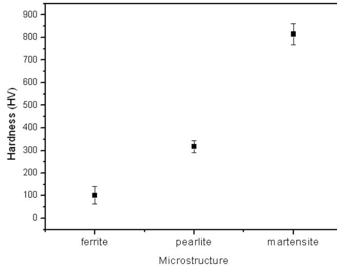
Figure 4. Results of Vickers hardness testing for the studied steels.
