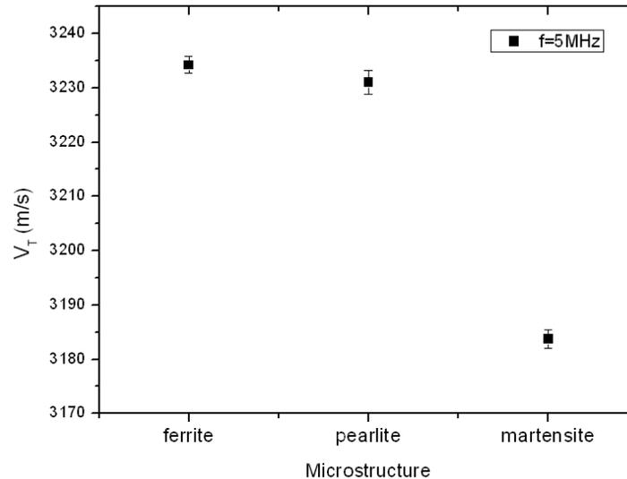
Figure 6. Correlation between microstructures and transversal ultrasonic velocities ( $V_T$ ) in the studied samples with a 5 MHz frequency.
