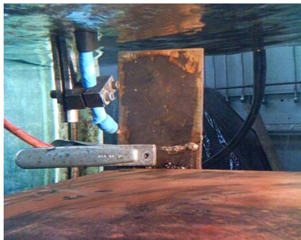
Figure 2. First view of the underwater initial trials in horizontal position (Copyright © TWI Ltd).
