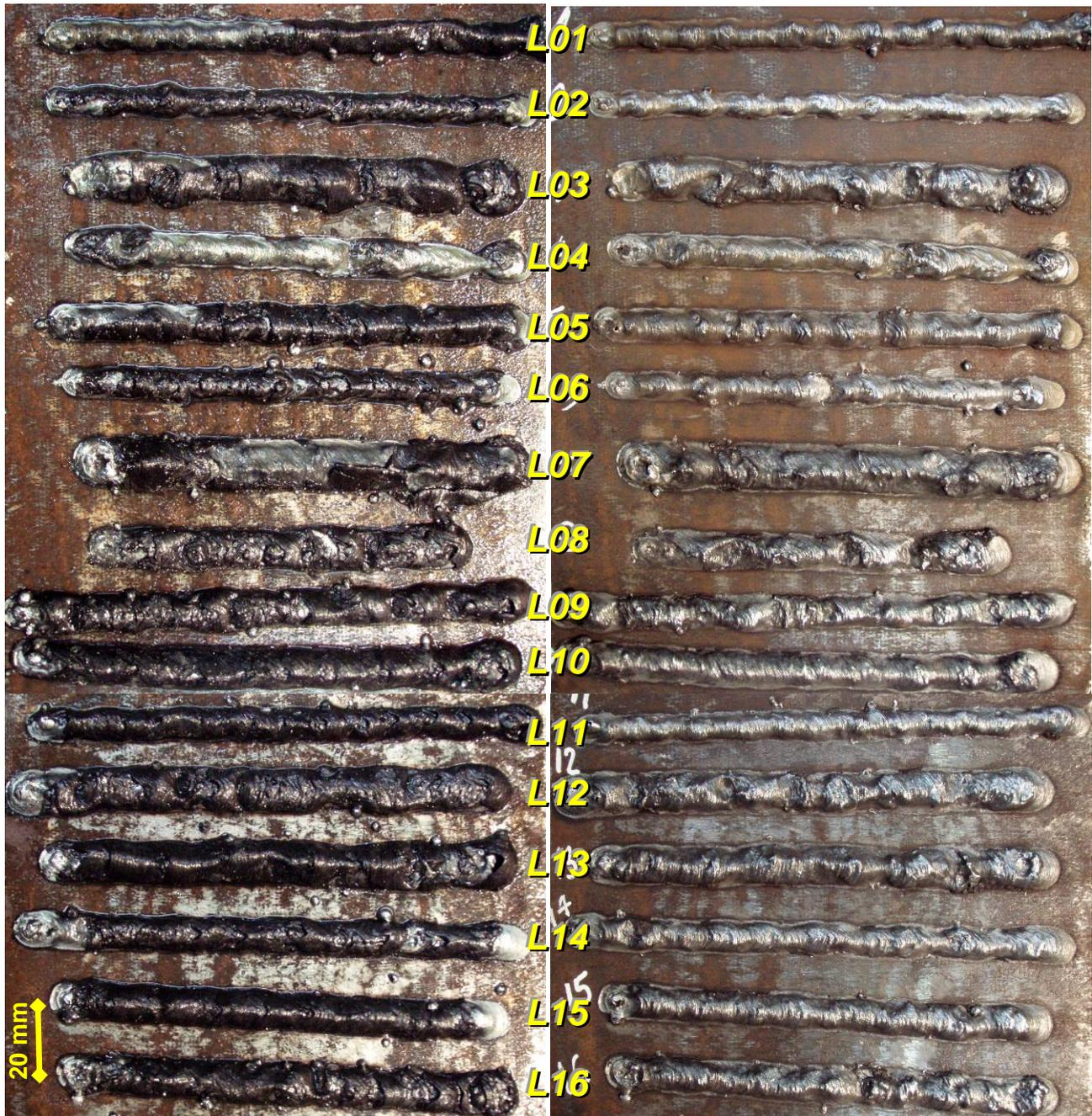
Figure 3. Bead appearance just after welding (left) and after manual brushing (right) (Copyright © TWI Ltd).
