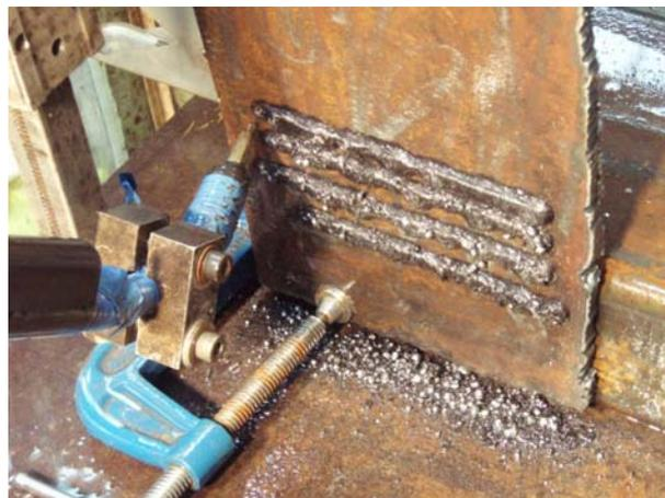
Figure 3. Large volume of spattering.
