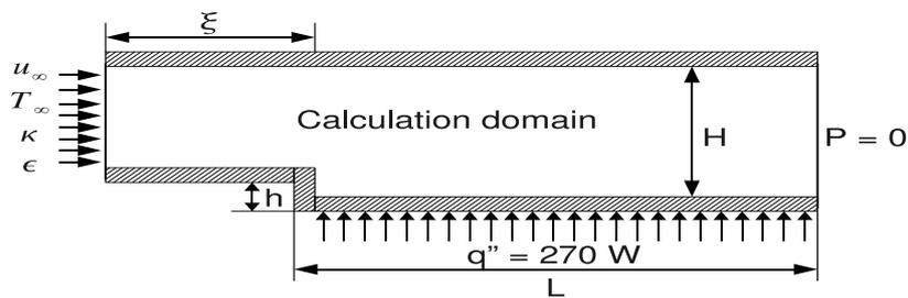
Figure 1. Calculation domain - Vogel and Eaton (1985) test case
