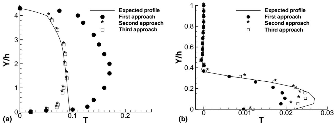
Figure 6. Temperature profiles in the asymmetric diffuser of Buice and Eaton (1995) -  $X/h=26$  (a) and in the 2D hill of Loureiro et. al (2007) in  $X/h=6.5$  (b)
