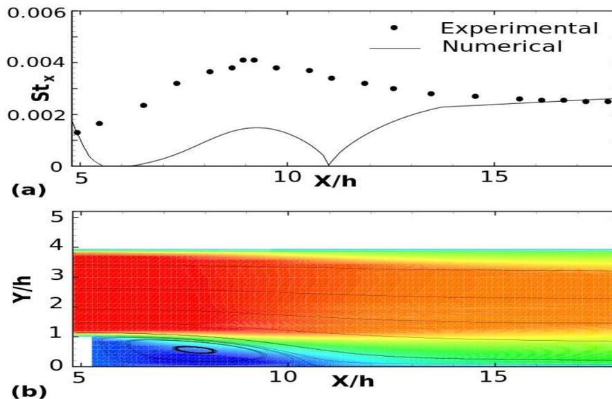
Figure 2. Numerical and experimental behavior of the Stanton number (a), velocity field and streamlines of the flow (b)
