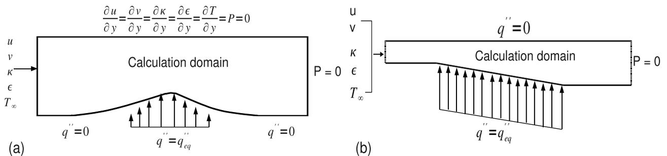
Figure 5. Geometry and boundary conditions of the Buice and Eaton (1995) diffuser (a), geometry and boundary conditions of the Loureiro et. al (2007) 2D hill (b)
