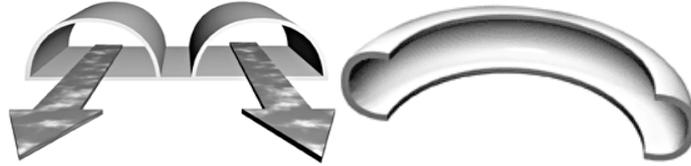
Figure 5: On the left schematic representation of the flow through the half-pipe coil; on the right, calendered profile of a half-pipe coil
