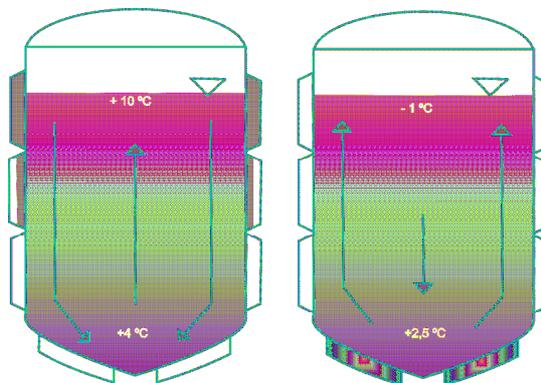
Figure 4: On the left, convection inside a CCV; on the right, cold storage of the beer (Kunze, 1999)
