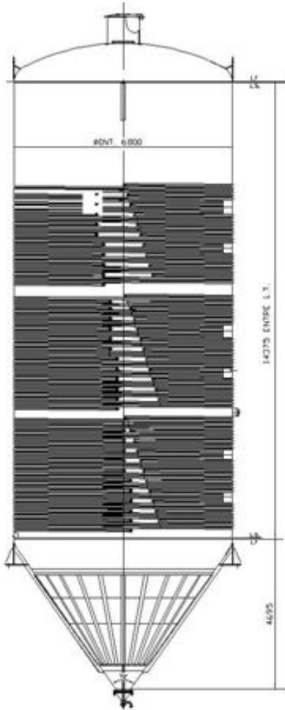
Figure 3: Cylindroconical fermenter
