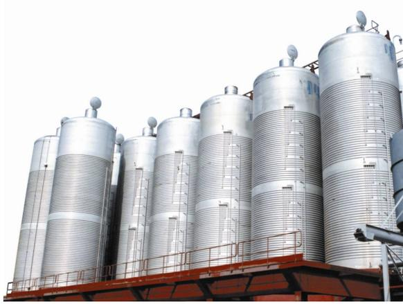
Figure 1: Cyindroconical fermenters still in assembly phase (without thermal isolation). DEDINI (2008)
