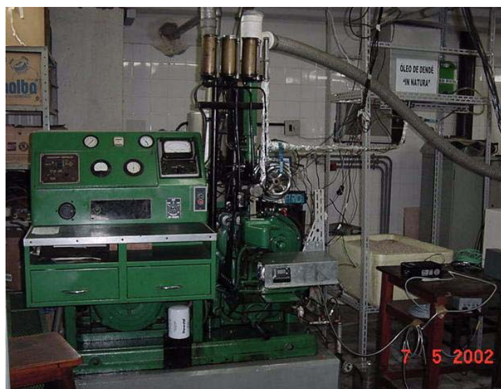
Figure 2. Test device –CFR Cetane Engine
