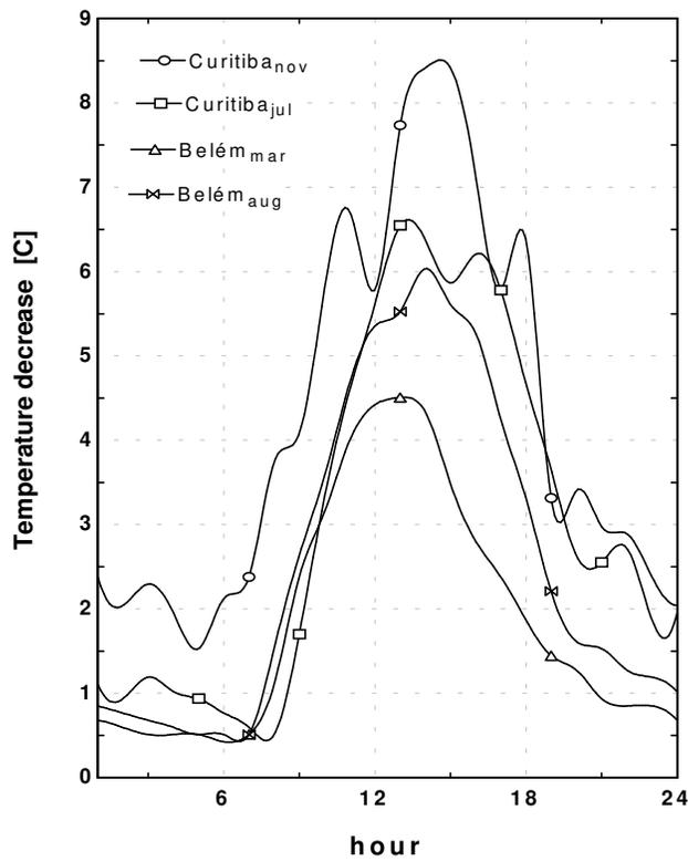
Figure 10 - Temperature decrease using EC in Belém and Curitiba.
