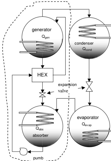
Figure 4 – Absorption cooling (AC) scheme.
