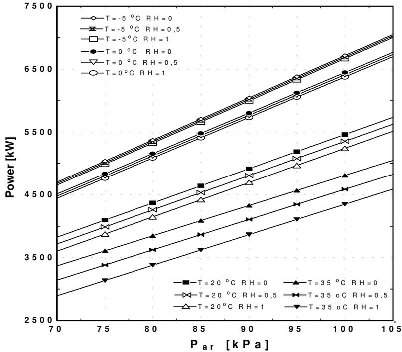
Figure 7 – Influence of inlet air pressure, temperature and relative humidity in the GT power.
