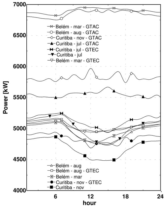
Figure 9 – Influence of the cooling-system in GT power during the day.
