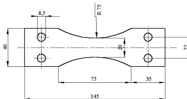
Figure 2. Specimens under study (dimension in mm).
