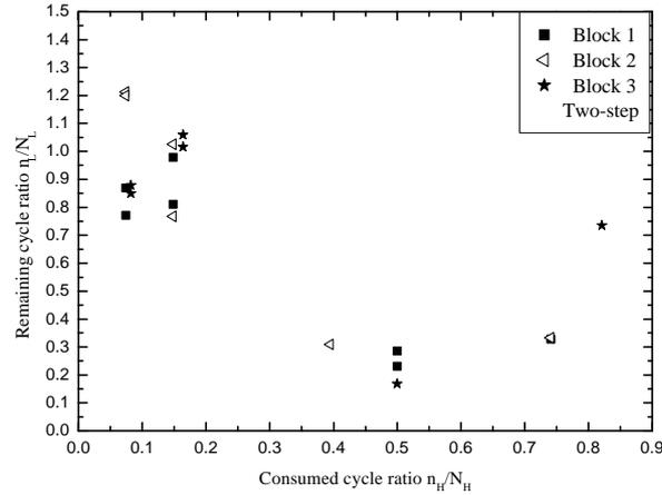
Figure 4. Effects of consumed cycles on the remaining cycle ratios for two-step.
