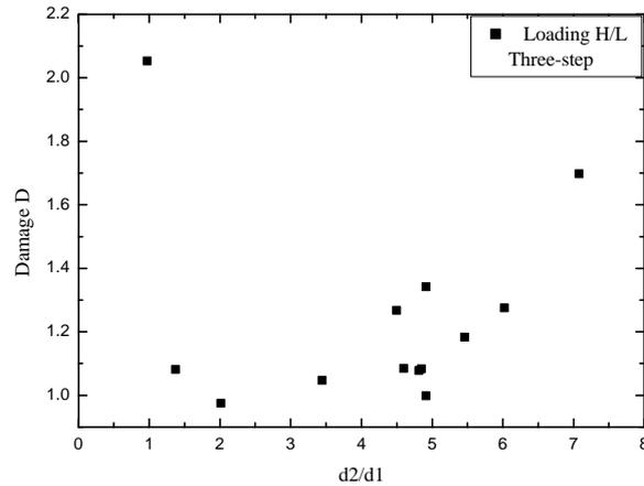
Figure 9. Correlation D versus  $d_2/d_1$  for three-step.
