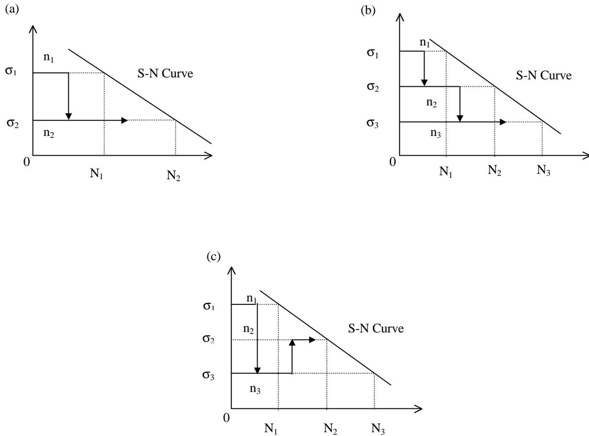
Figure 3. Block program loading. (a) two-step, (b) three-step and (c) three-step alternate.
