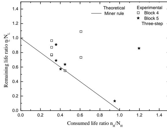
Figure 8. Correlation between theoretical predictions and experimental results for three-step.
