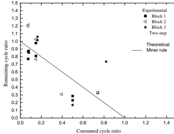
Figure 6. Correlation between theoretical predictions and experimental results for two-step.
