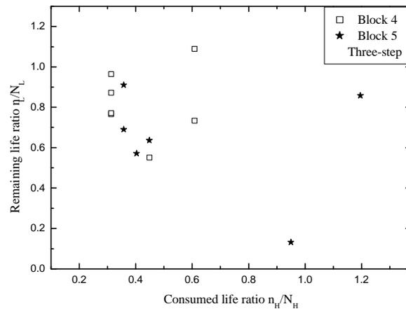
Figure 5. Effects of consumed cycles on the remaining cycle ratios for three-step.
