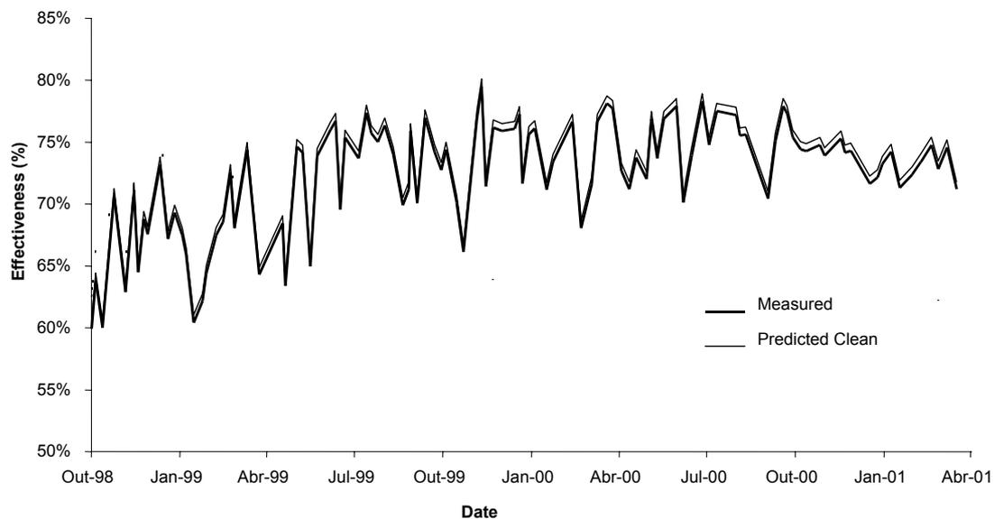
Figure 2. Comparison of the measured and predicted clean effectiveness of HX-04.
