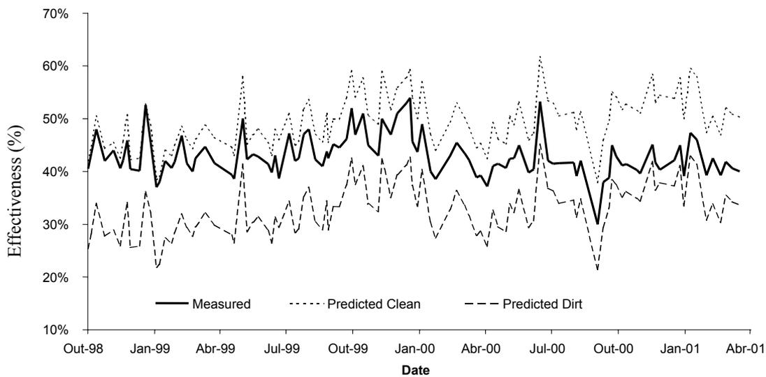
Figure 5. Comparison of the measured and predicted clean and dirt effectiveness of HX-03.
