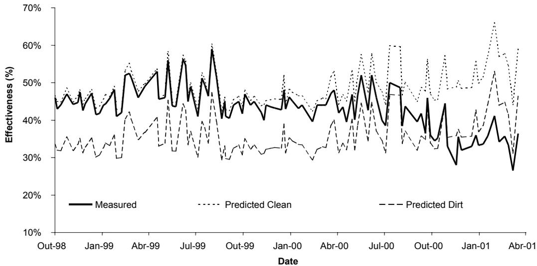
Figure 3. Comparison of the measured and predicted clean and dirt effectiveness of the HX-01.
