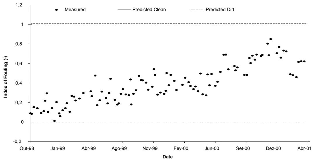
Figure 6. Index of fouling for the HX-03.
