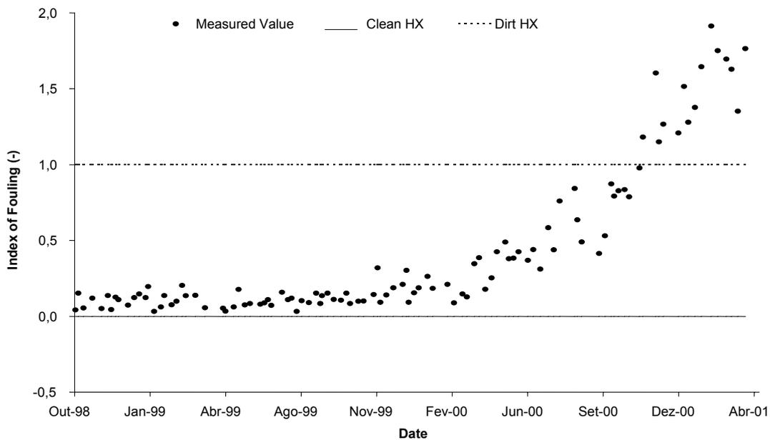
Figure 4. Index of fouling for the HX-01.
