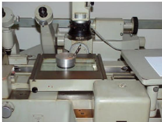
Figure 6. Wear measurements of the drills using a microscope JENA 3313.
