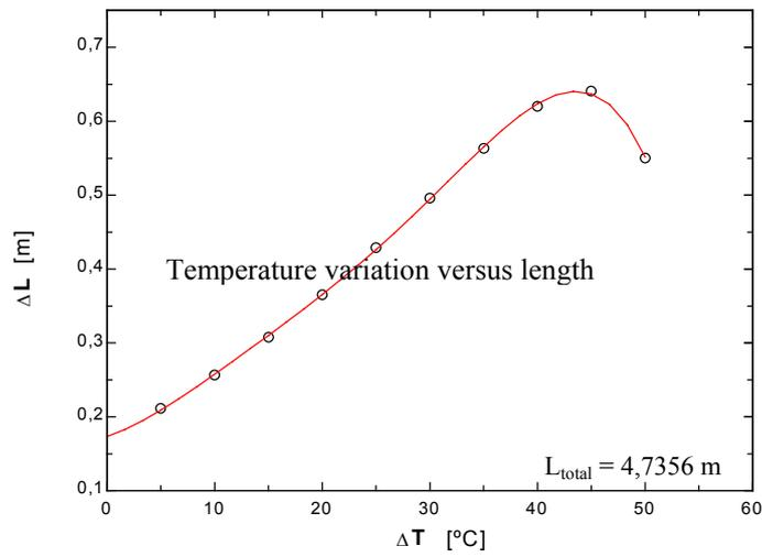
Figure 3. Temperature variation versus length of the capillary tube to each section with temperatures varying in 5°C and using diameter of 0,8mm.
