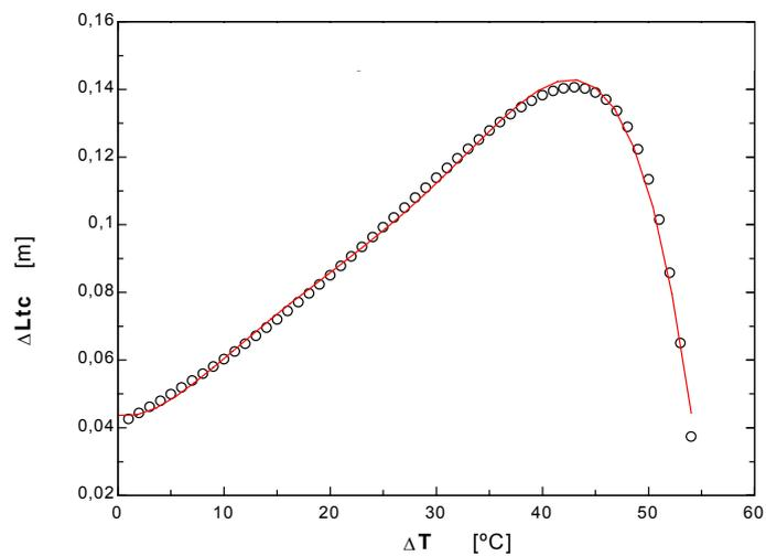
Figure 5. Temperature variation versus length variation of the capillary tube to each section, with temperatures varying in 1°C and using diameter of 0,6mm.
