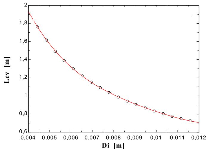
Figure 2. Diameter versus length of the evaporator tube
