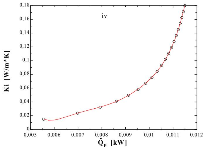
Figure 7. Thermal Conductivity of the isolation versus heat transfer rate.
