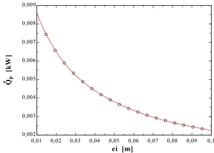
Figure 6. Heat transfer rate of the walls versus thickness of the insulating.
