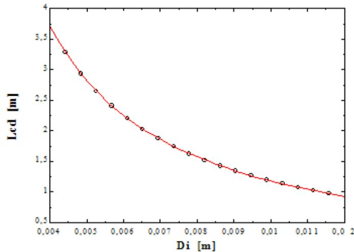
Figure 1. Diameter versus length of the condenser tube.
