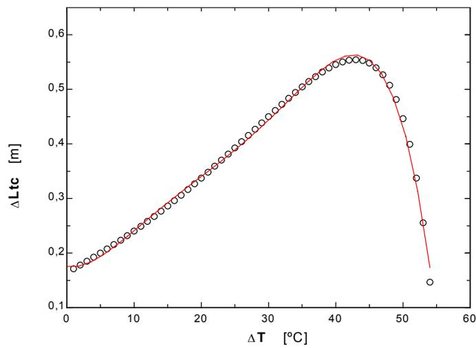
Figure 4. Temperature variation versus length of the capillary tube to each section with temperatures varying in 1°C and using diameter of 0,8mm
