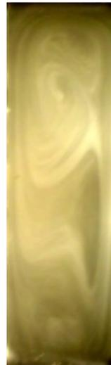
Figure 13. Flow visualization with smoke tracing technique, for the basic case considered (case 2).
