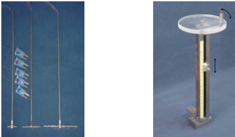
Figure 4. Thermocouple probes and positioning system for temperature measurements inside the cavities.
