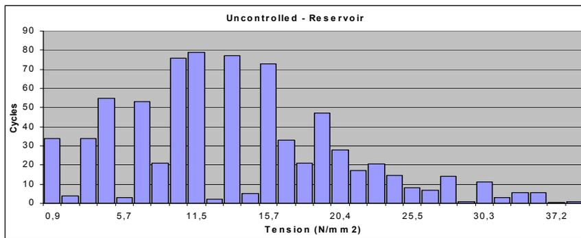
Figure 5b- Histogram – number of cycles x tension – **Reservoir** Method – **uncontrolled** system
