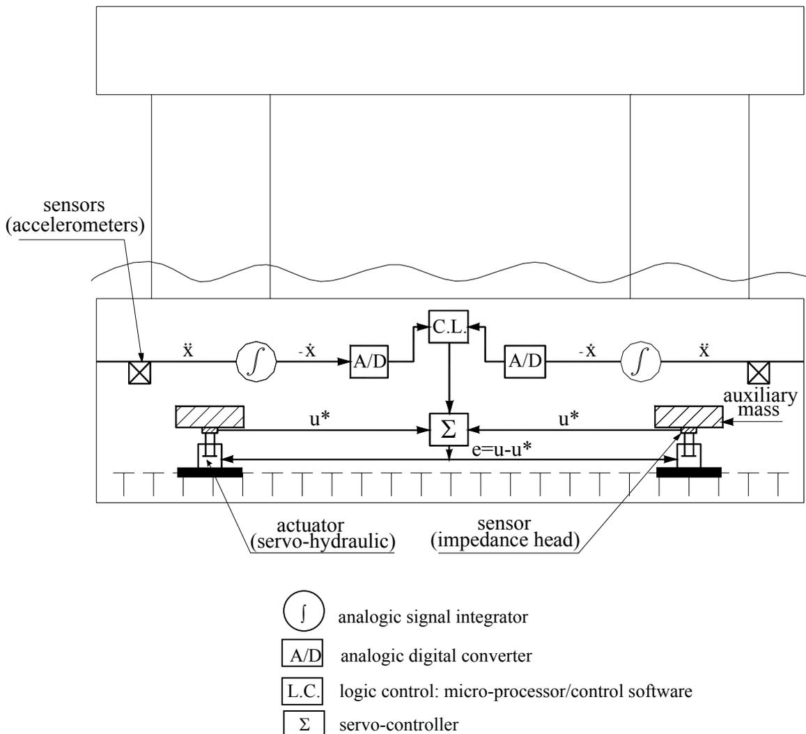
Figure 2 - Schematic of active control in TLP
