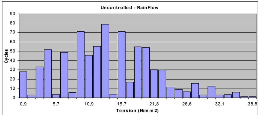
Figure 5a- Histogram – number of cycles x tension – **Rainflow** Method – **uncontrolled** system
