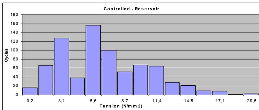
Figure 5d - Histogram – number of cycles x tension – **Reservoir** Method – **controlled** system
