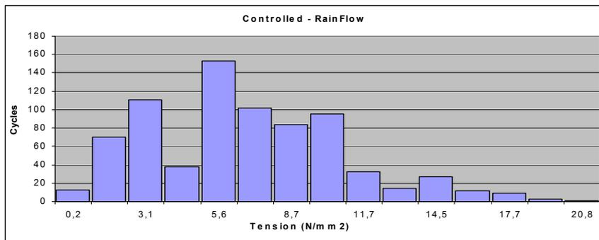
Figure 5c - Histogram – number of cycles x tension – **Rainflow** Method – **controlled** system
