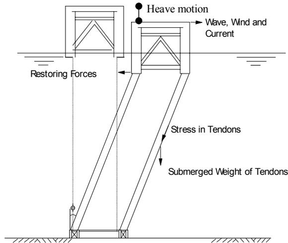
Figure 1. Environmental load under TLP
