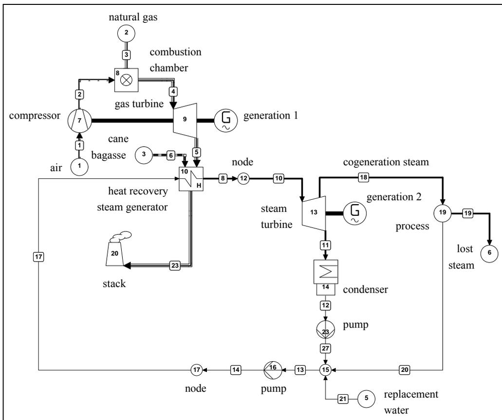
Figure 4. System A with a heat recovery steam generator that burns sugar cane bagasse with the exhaust gases of the gas turbine (**System D**).
