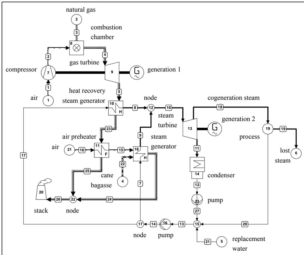
Figure 3. System B, with boiler air preheater (**System C**).
