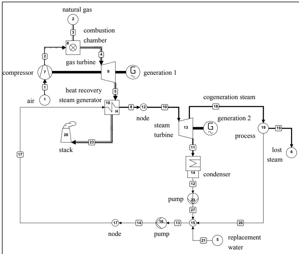
Figure 1. Combined cycle based system with cogeneration using only natural gas (**System A**).
