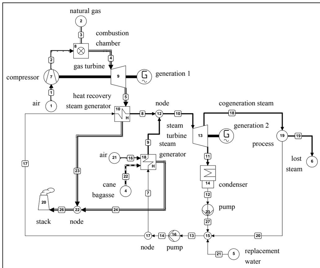
Figure 2. System A with another steam generator that uses sugar cane bagasse (**System B**).
