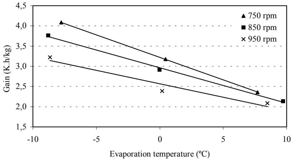
Figure 5 – Evolution of the gain of the evaporator in function of the evaporation temperature.
