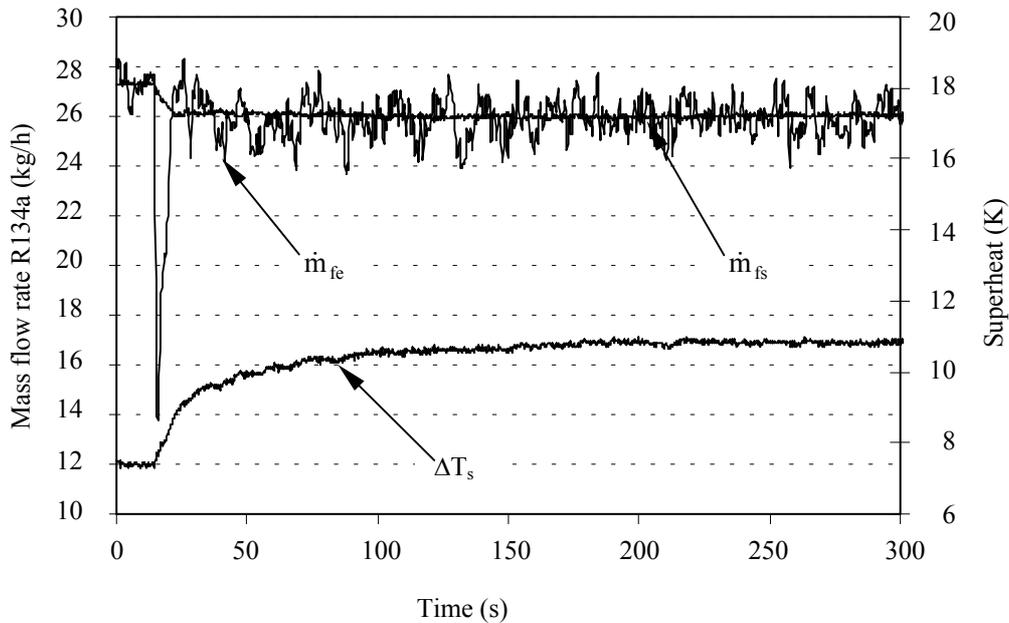
Figure 3 - Response of the degree of superheating to a perturbation of the step type on the mass flow of the refrigeration fluid
