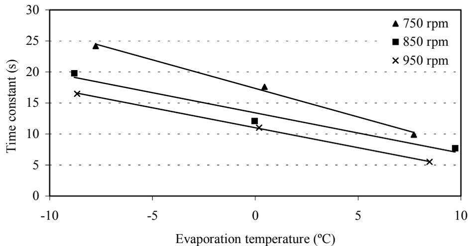
Figure 6 – Evolution of the time constant of the evaporator in function of the evaporation temperature.
