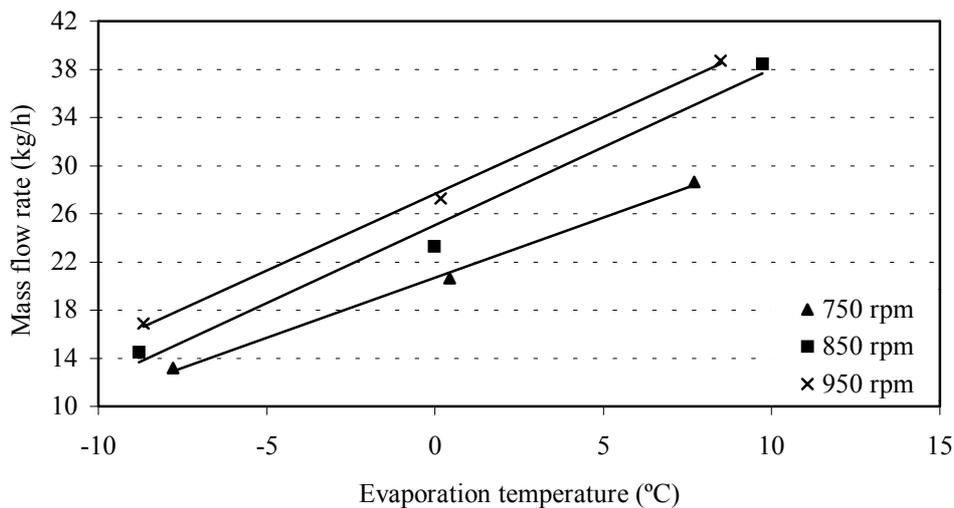
Figure 4 – Evolution of the mass flow rate in function of the evaporation temperature and the compressor speed.
