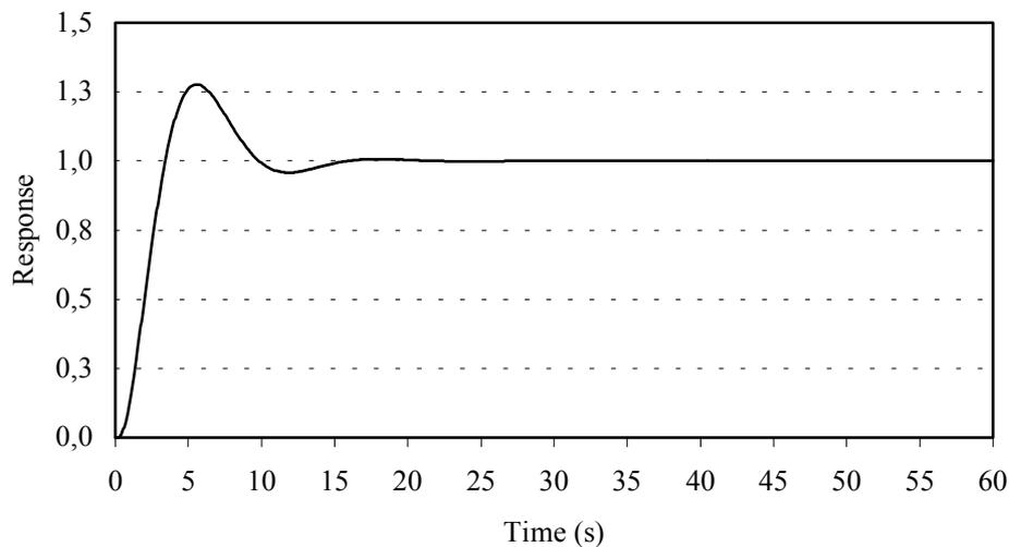
Figure 7 – Response of the control system of the step increase of the superheating in the evaporator in a closed loop to a unitary step at the inlet for  $T_{cb} = 10^{\circ}\text{C}$  and  $N = 950$  rpm.
