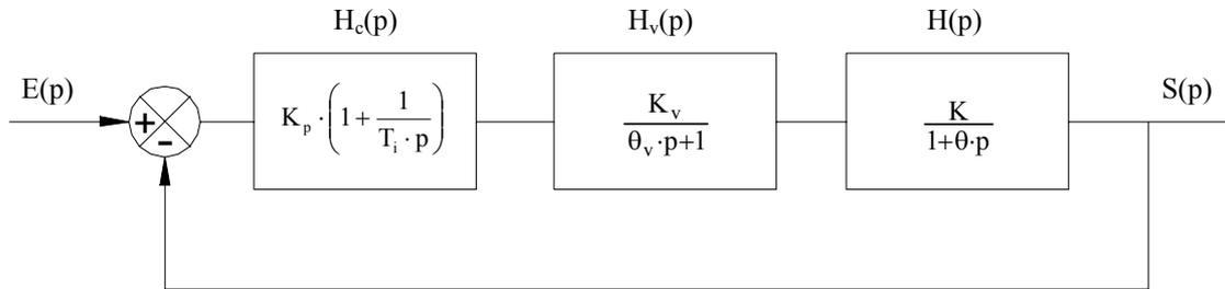
Figure 2 – Representation by a block diagram of the control system of the evaporator
