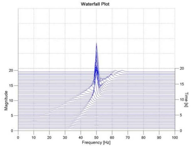
Figure 15. Waterfall Plot of isotropic rotor with two crossing orders.
