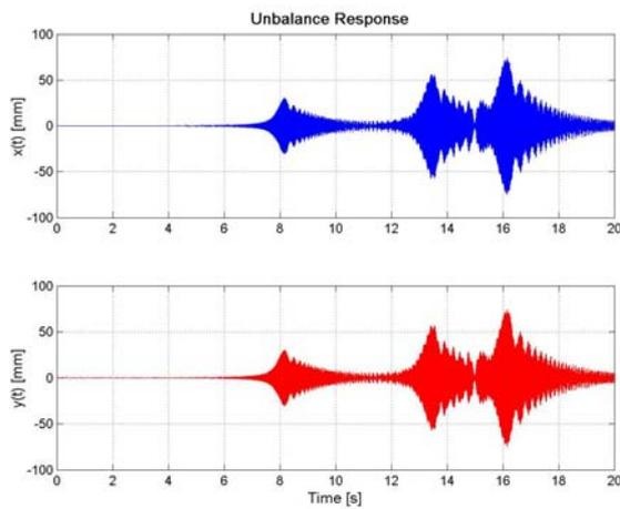
Figure 20. Unbalance response of isotropic rotor.
