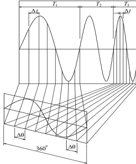
Figura 2. Angular domain representation of a signal.
