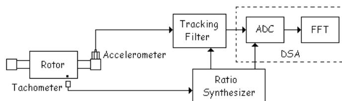
Figure 1. Analog order tracking method.
