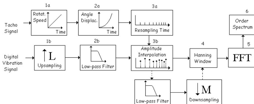
Figure 4. Steps in the digital resampling method.
