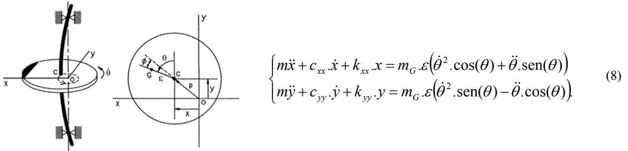
Figure 5. DeLaval rotor system and equations of motion.
