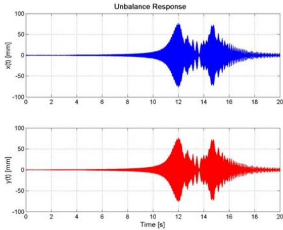
Figure 14. Unbalance response of isotropic rotor with two crossing orders.
