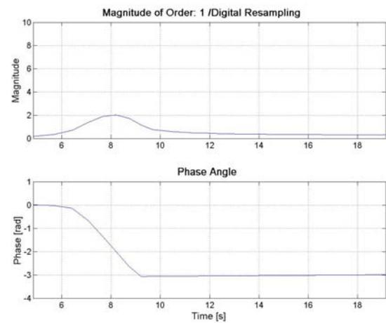
Figure 11. Magnitude and phase. Digital resampling.
