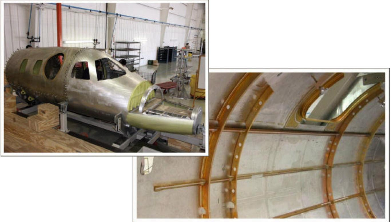
Figure 7. Eclipse 500 Final Assembly and Entirely FSW Panel (Velocci, 2000)
