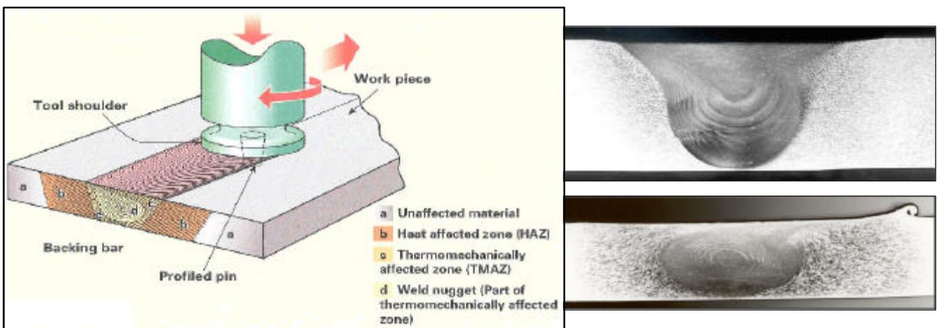
Figure 3. FSW Transverse macrosection (adapted from Threadgill, 2002)
