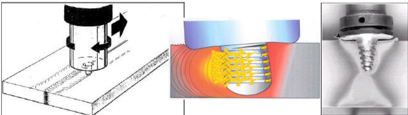
Figure 1. Schematic Friction Stir Welding Principle (adapted from Threadgill , 2002; and Kalle, 2002 )
