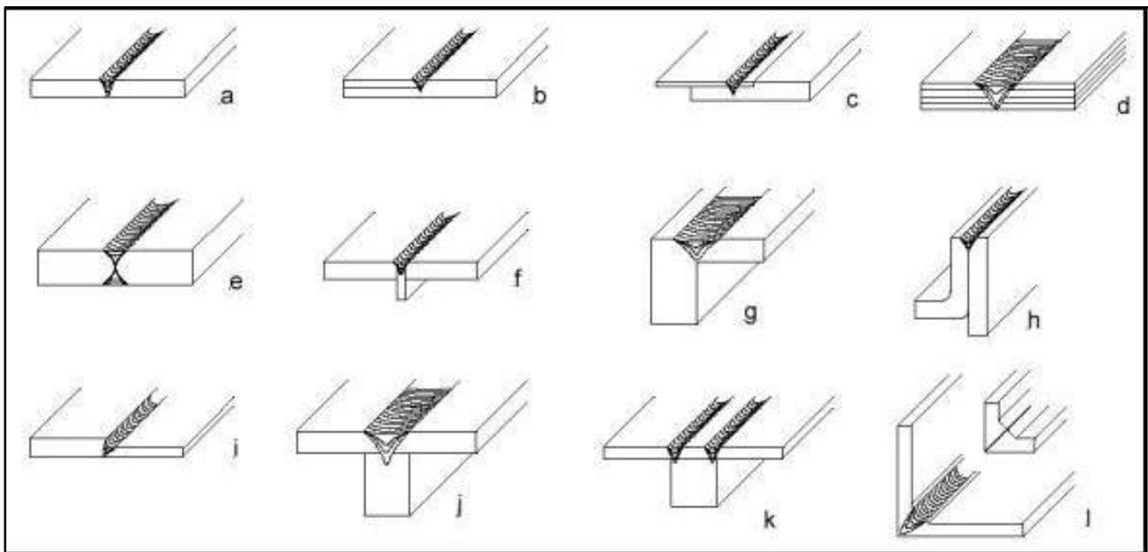
Figure 4. Typical Joint Designs for Friction Stir Welding (adapted from Threadgill, 2002).
