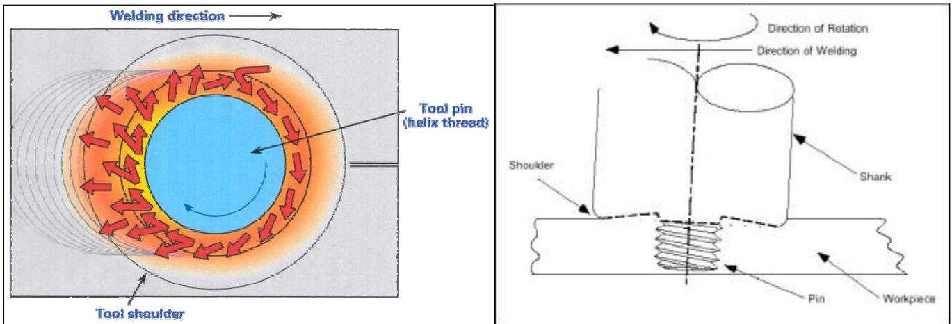
Figure 2. Schematic Friction Stir Welding Principle (adapted from Threadgill, 2002; and Reynolds, 2000)
