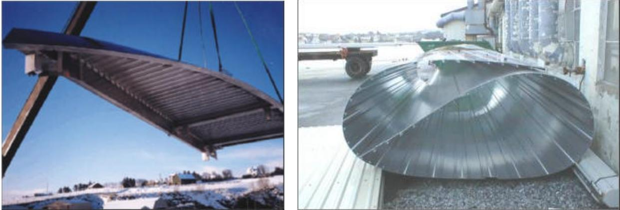
Figure 5. Prefabricated FSW Panel for Naval Applications (Midling, 1999)
