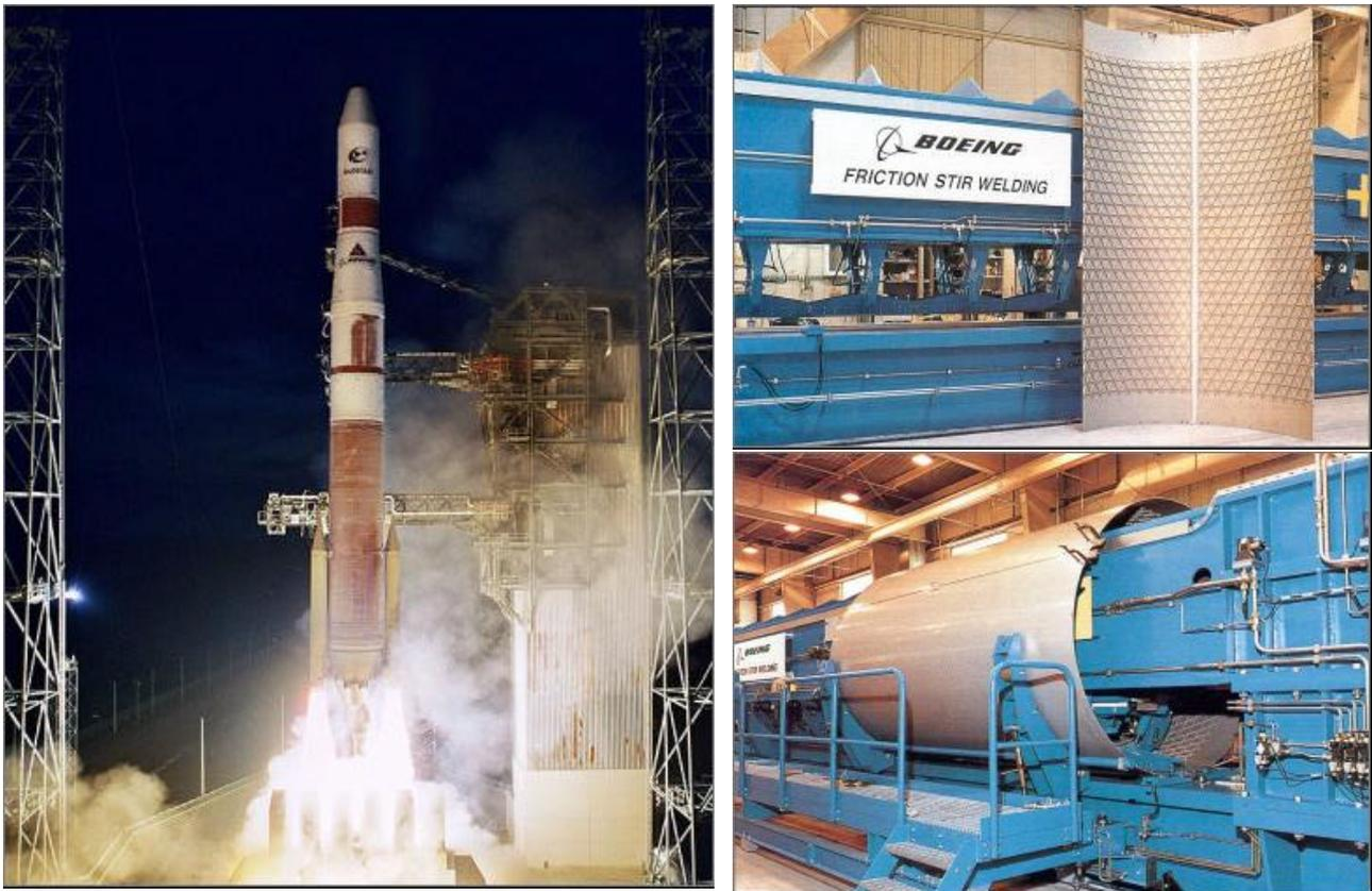
Figure 6. Delta IV Rocket and its FSW Tank Manufacturing (Boeing website)
