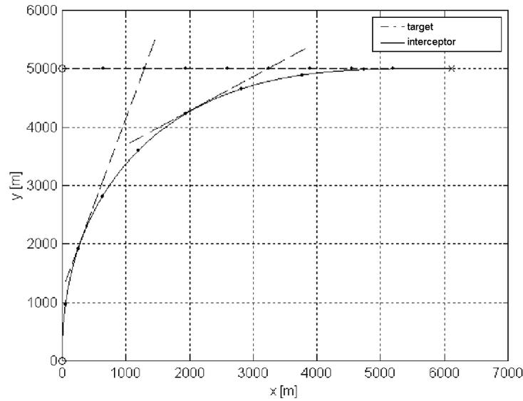
Figure 2: target and interceptor trajectories for a velocity pursuit intercept
