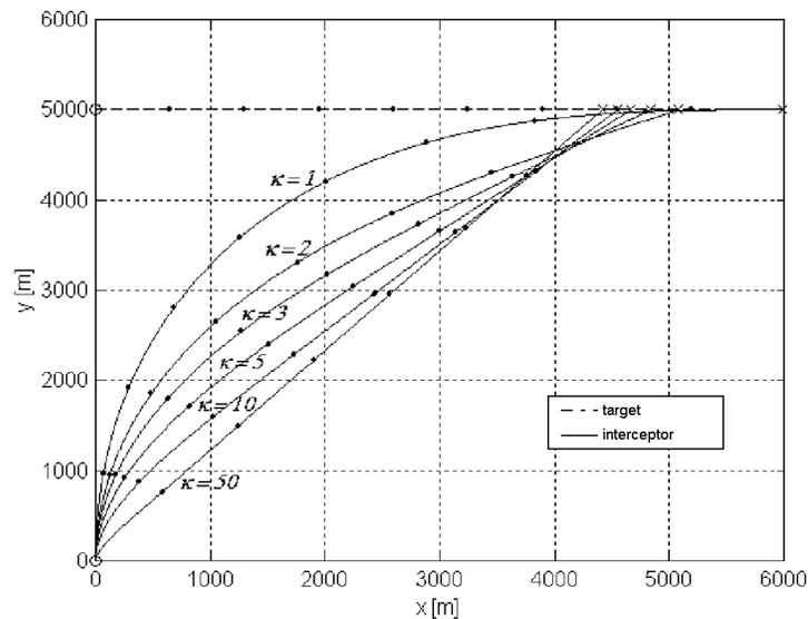
Figure 3: target and interceptor trajectories for several navigation constants ruled by PNG
