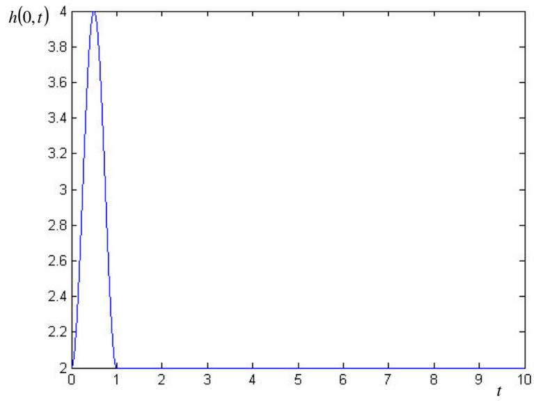
Figure 5.2. Boundary condition for the height of water at  $x = 0$ .
