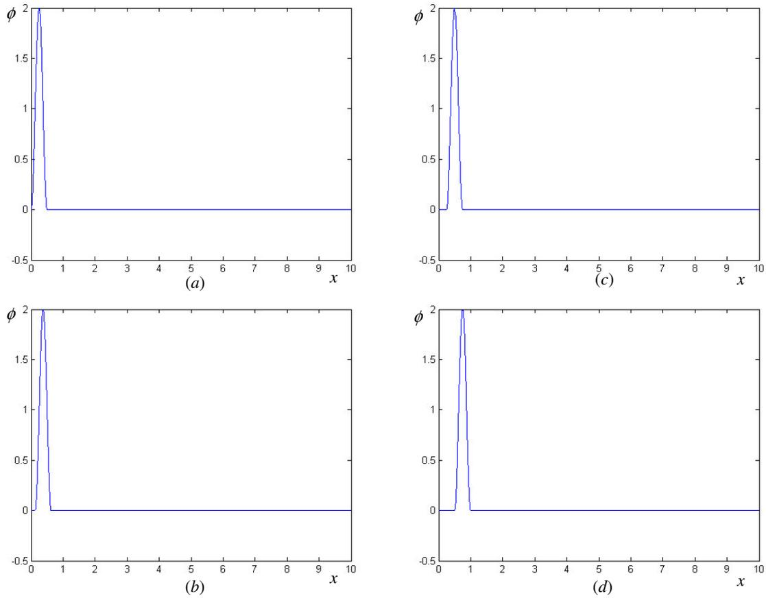
Figure 5.1. Evolution of pollutant concentration profile with constant velocity and water height: (a)  $t = 0$ ; (b)  $t = 1/4$  day; (c)  $t = 1/2$  day; (d)  $t = 1$  day.
