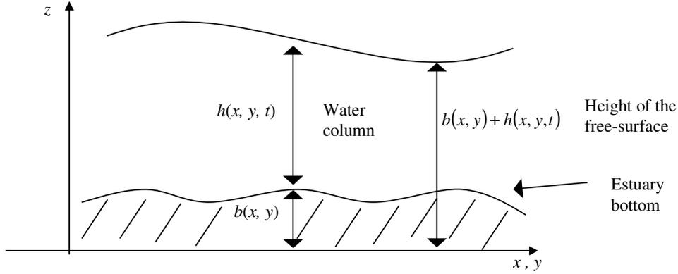
Figure 2.1. Representation of a free-surface flow in an estuarine region.
