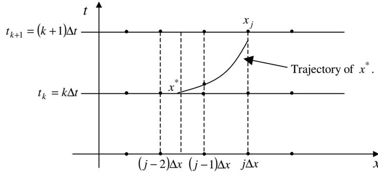
Figure 4.1. Time advancing of  $\phi$  through the characteristics.
