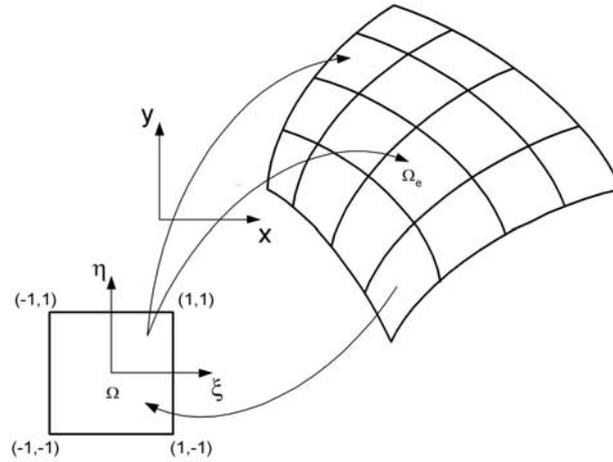
Figure 2. Representation of the isoparametric element.
