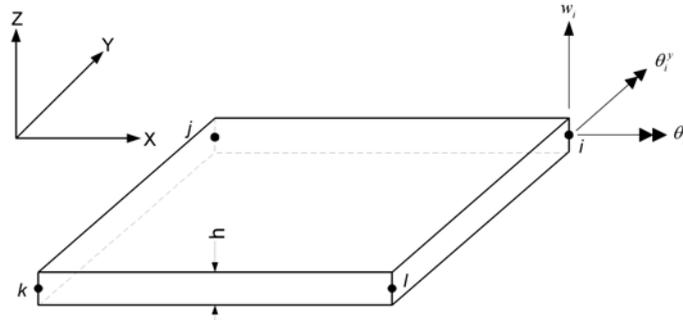
Figure 1. Nodal displacement for four node plate element.
