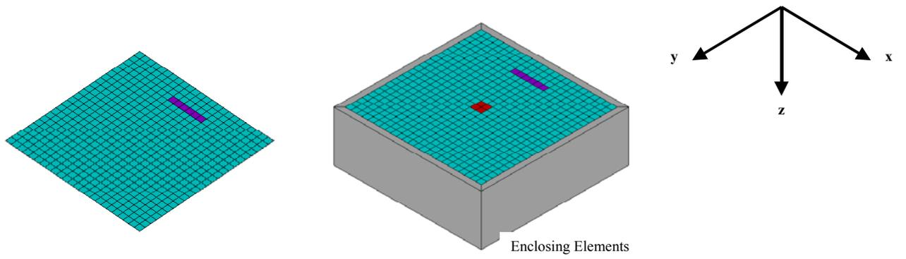
a) Discretization of the soil free surface and barrier
