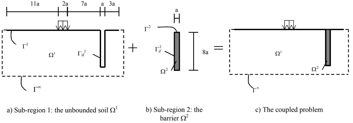
Figure 1: Lateral view of the unbounded soil and the bounded barrier
