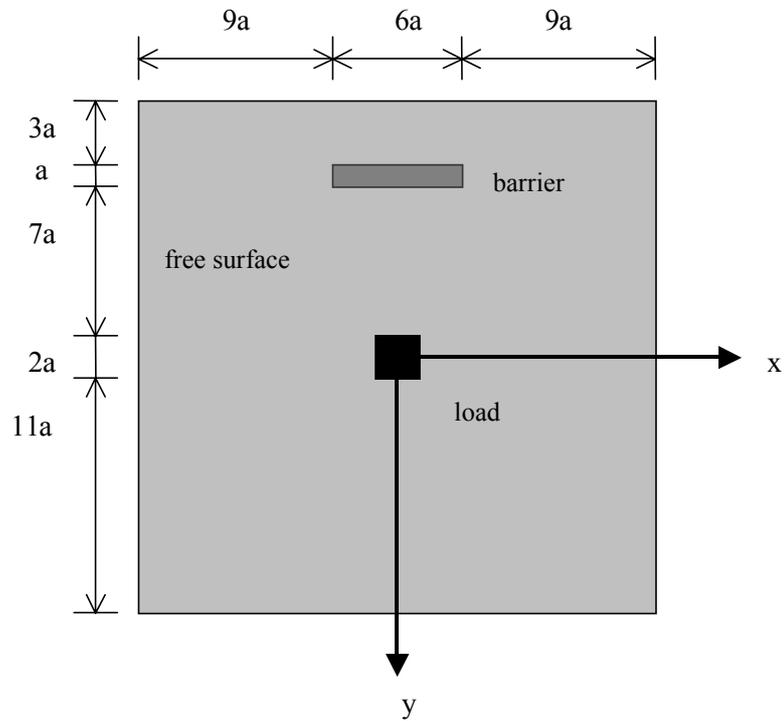
Figure 3: Scheme for the dimensions and position of the soil free surface, loaded area and barrier.
