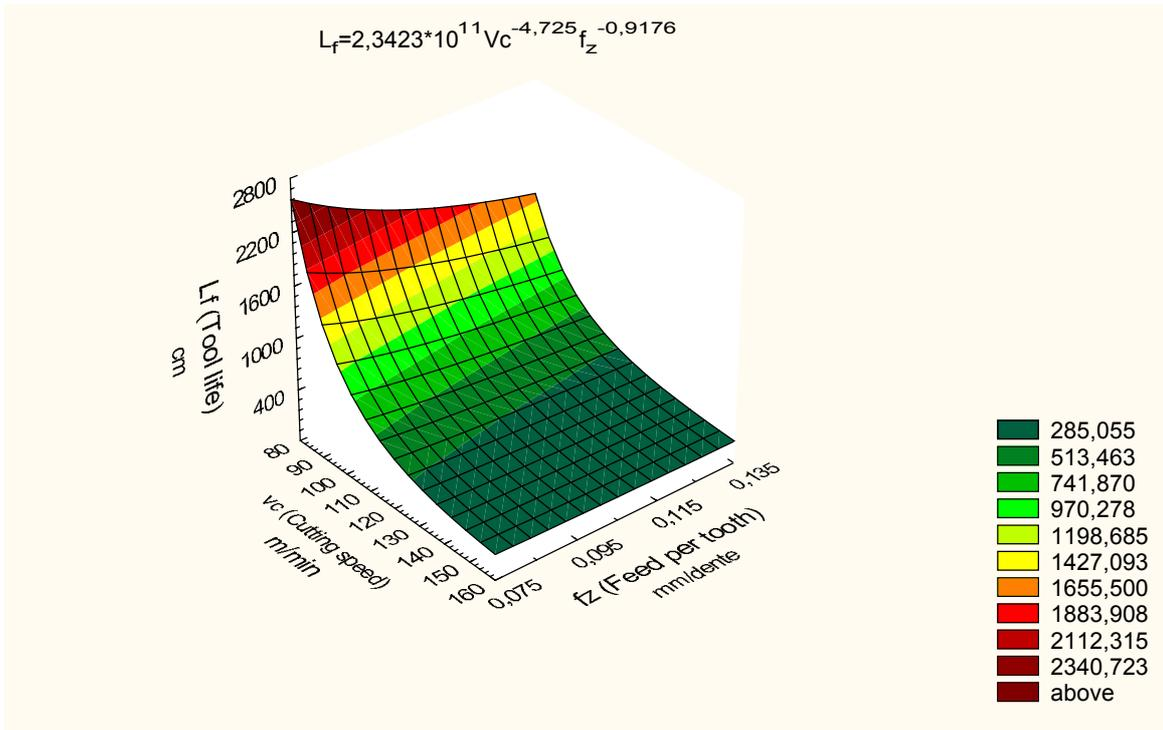
Figure 6. Response surface adjusted to tool life, related to the depth of cut of 1.00 mm.
