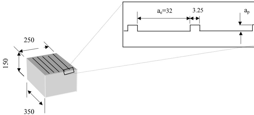
Figure 2. Basic geometry of the test block and the slot milling process
