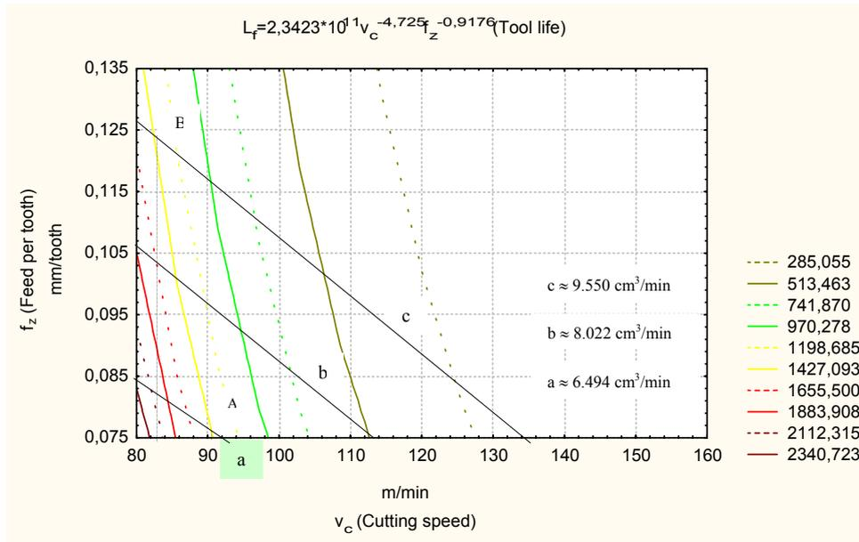
Figure 4. Tool life bound and MRR (cm<sup>3</sup>/min) in cutting speed-feed per tooth plane for cut depth of 1.00 mm
