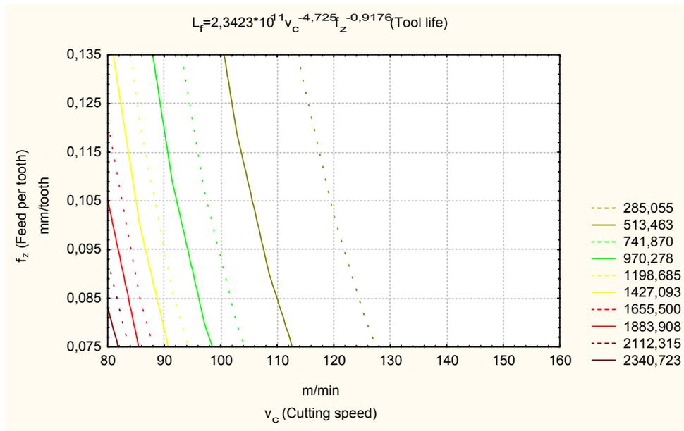
Figure 3. Bound of tool life in cutting speed-feed per tooth plane for depth of cut of 1.00mm.
