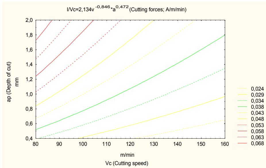
Figure 5. Cutting force bound in cutting speed plane for a feed per tooth of 0.1mm/tooth.
