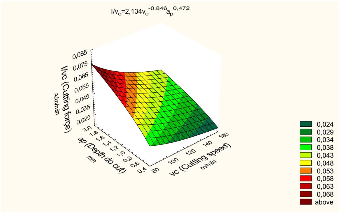
Figure 7. Response surface adjusted to cutting force, related to the feed per tooth of 0.10 mm/tooth.
