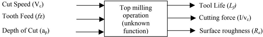
Figure 1 – Relation between the input factors and the observed output response
