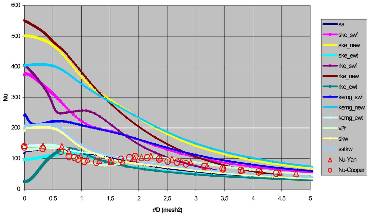
Figure 4. Nusselt distribution along radial distance for mesh 2.
