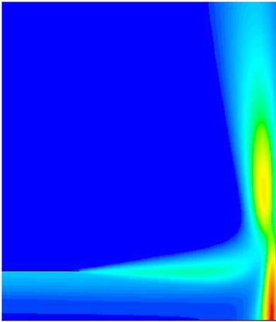
Figure 7. Contours of  $k$  (turbulent kinetic energy) – Standard  $k-\epsilon$  with standard wall function.
