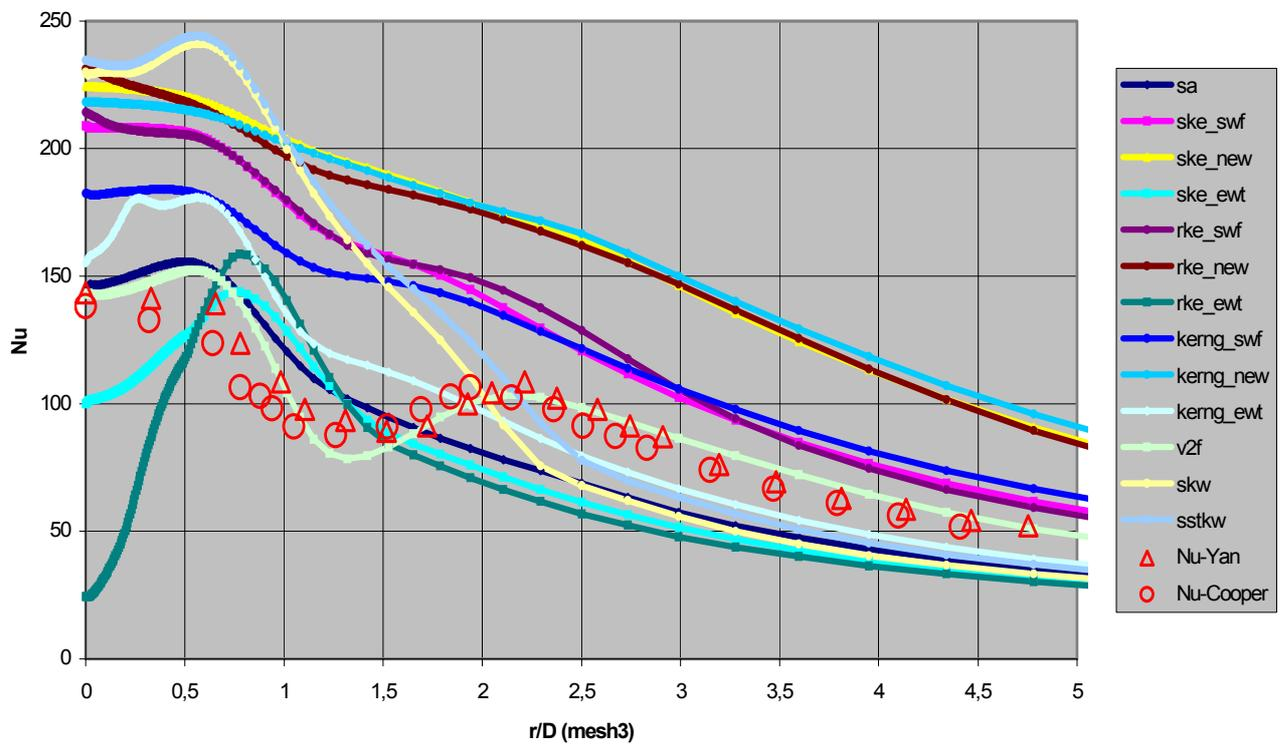
Figure 5. Nusselt distribution along radial distance for mesh 3.
