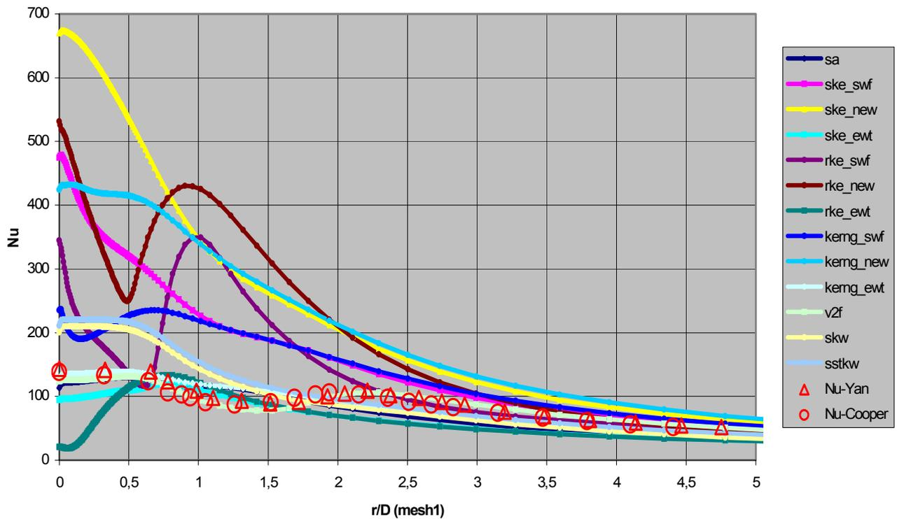
Figure 3. Nusselt distribution along radial distance for mesh 1.
