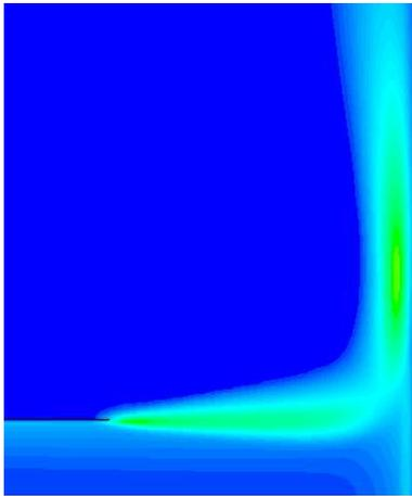
Figure 9. Contours of  $k$  (turbulent kinetic energy) –  $k-\epsilon$  RNG with enhanced wall treatment.
