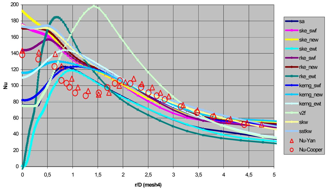
Figure 6. Nusselt distribution along radial distance for mesh 4.
