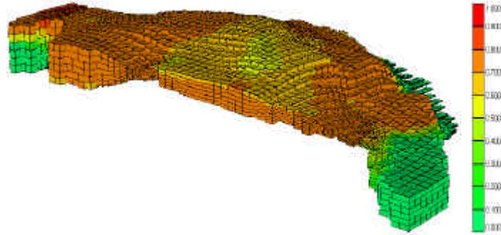
Figure 1: Simulation model of the reservoir. The legend indicates the oil saturation.
