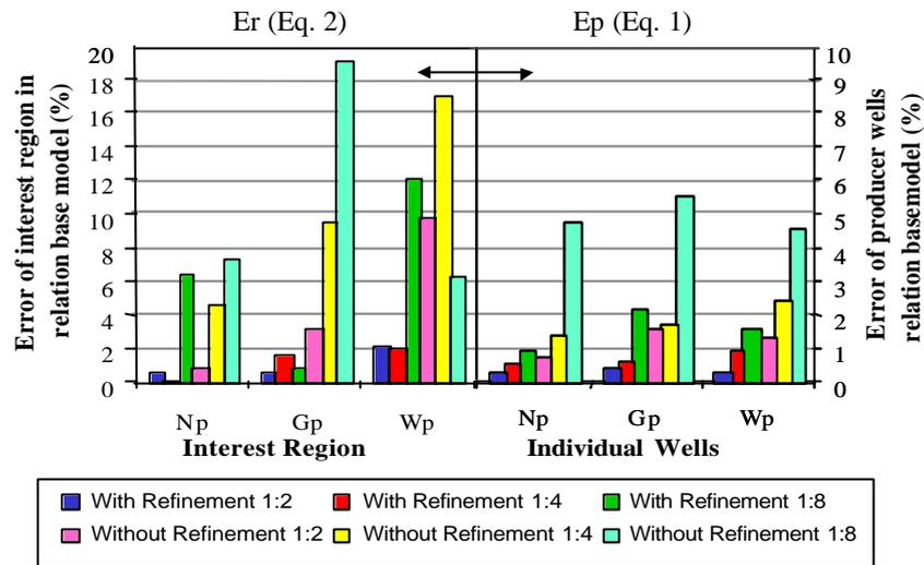
Figure 8: Errors in the cumulative productions for models with and without refinement in relation to the base model.
