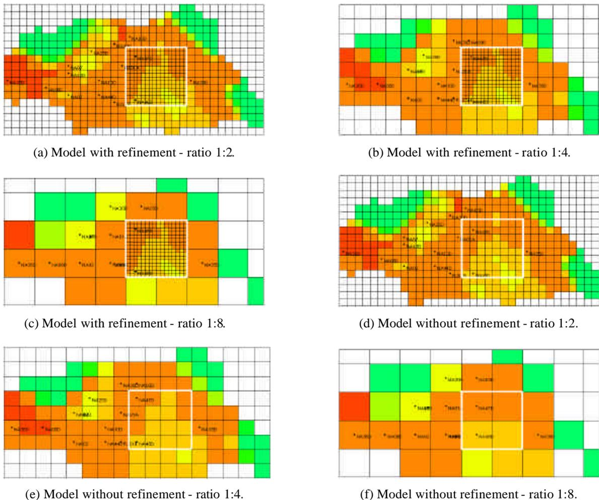
Figure 6: Different meshes for the evaluation of the effect of refinement.
