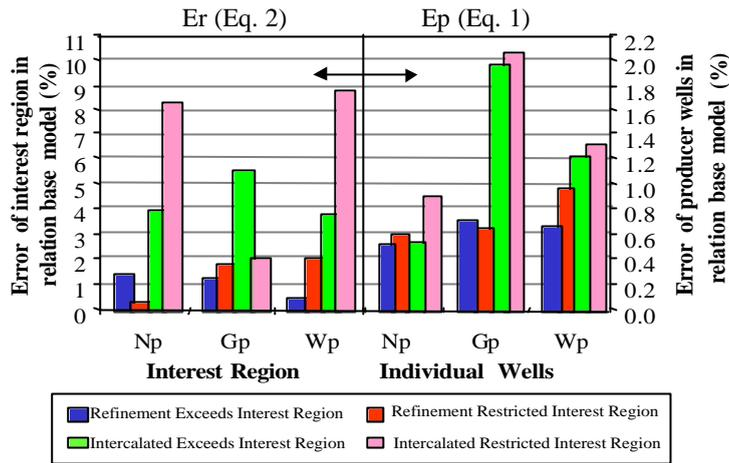
Figure 5: Errors in the cumulative productions in comparison with the base model, for each type of refinement.
