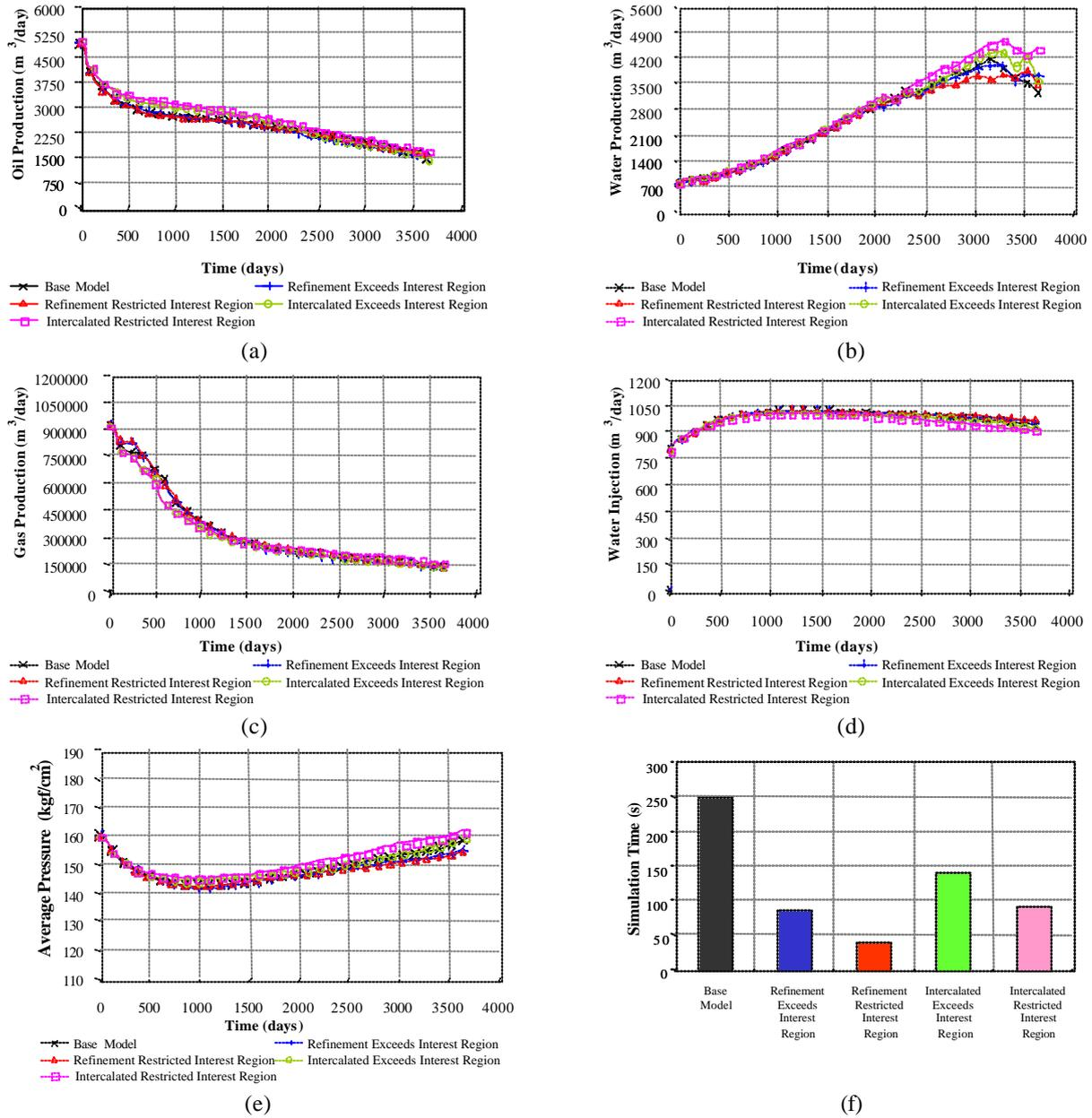
Figure 4: Oil Production (a), Water Production (b), Gas Production (c), Water Injection (d), Average Pressure (e) and Simulation Time (f) after ten years of forecast, for different type and localization of the refinement.
