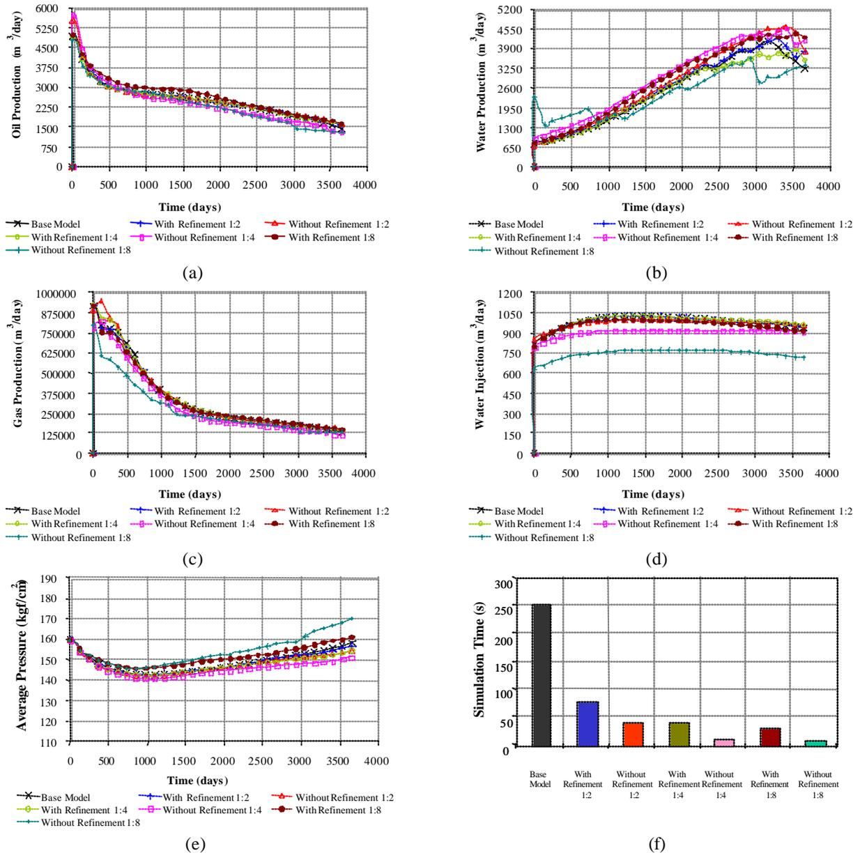
Figure 7: Oil Production (a), Water Production (b), Gas Production (c), Water Injection (d), Average Pressure (e) and Simulation Time (f) after ten years of forecast, for evaluation of the effect of refinement.
