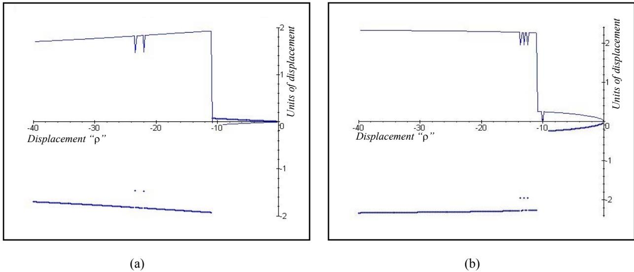
Figure 5a. Crack shape under an external loading,  $K_e$ , equals to the internal loading imposed by the dislocation,  $K_d$  – both sides; 5b –  $K_e$  is 2.4 times greater than the loading imposed by the dislocation  $K_d$  – both sides, (Bissa, 2002).
