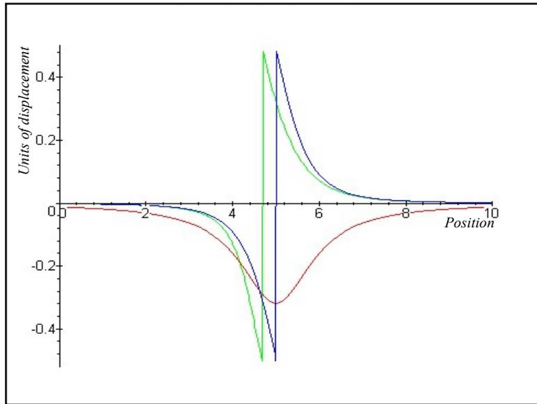
Figure 3. Superposition of displacement curves on the free surface of a semi-infinite medium.  $u_x$  (blue curve),  $u_y$  (red curve) and  $u_x$  and  $u_y$  (green curve), (Bissa, 2002).
