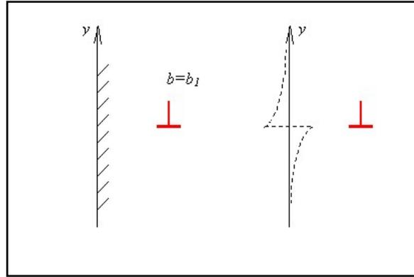
Figure 1. Schematic displacement due to the presence of a dislocation in a semi-infinite medium.
