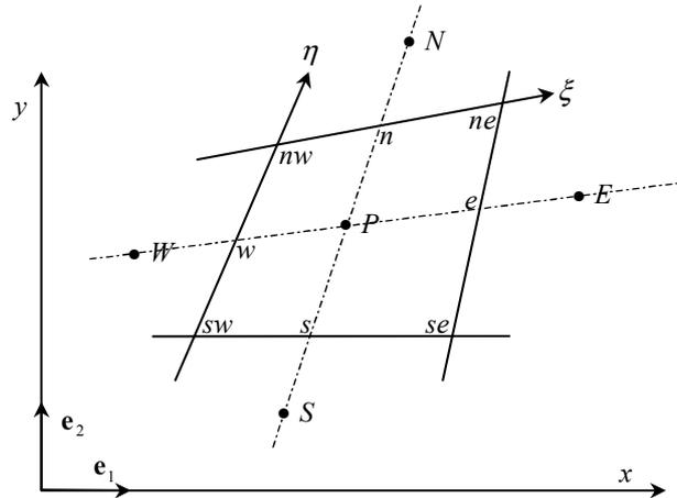
Figure 2: Notation for control volume discretization.
