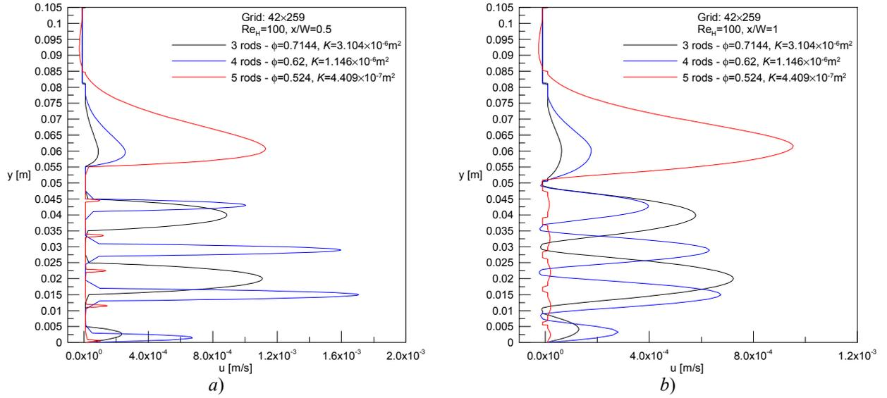
Figure 6: Effect of the porosity,  $\phi$ , in the velocity fields for  $H=0.08\text{m}$ : a) section at  $x/W=0.5$ ; b) section at  $x/W=1$
