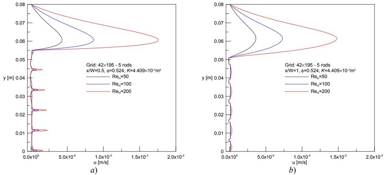
Figure 3: Effect of Reynolds number for  $H=0.08\text{m}$ : a) section at  $x/W=0.5$ ; b) section at  $x/W=1$ .
