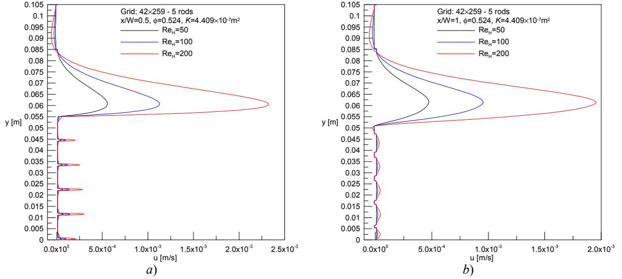
Figure 5: Effect of Reynolds number for  $H=0.105\text{m}$ : a) section at  $x/W=0.5$ ; b) section at  $x/W=1$ .
