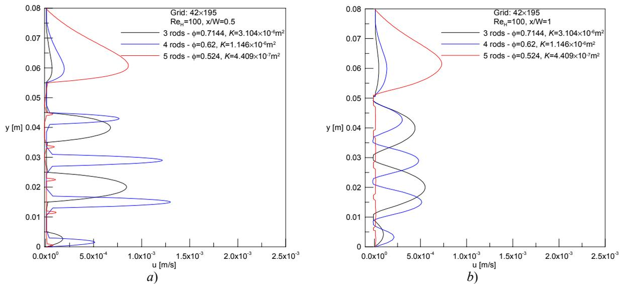
Figure 4: Effect of porosity,  $\phi$ , in the velocity fields for  $H=0.08\text{m}$ : a) section at  $x/W=0.5$ ; b) section at  $x/W=1$ .
