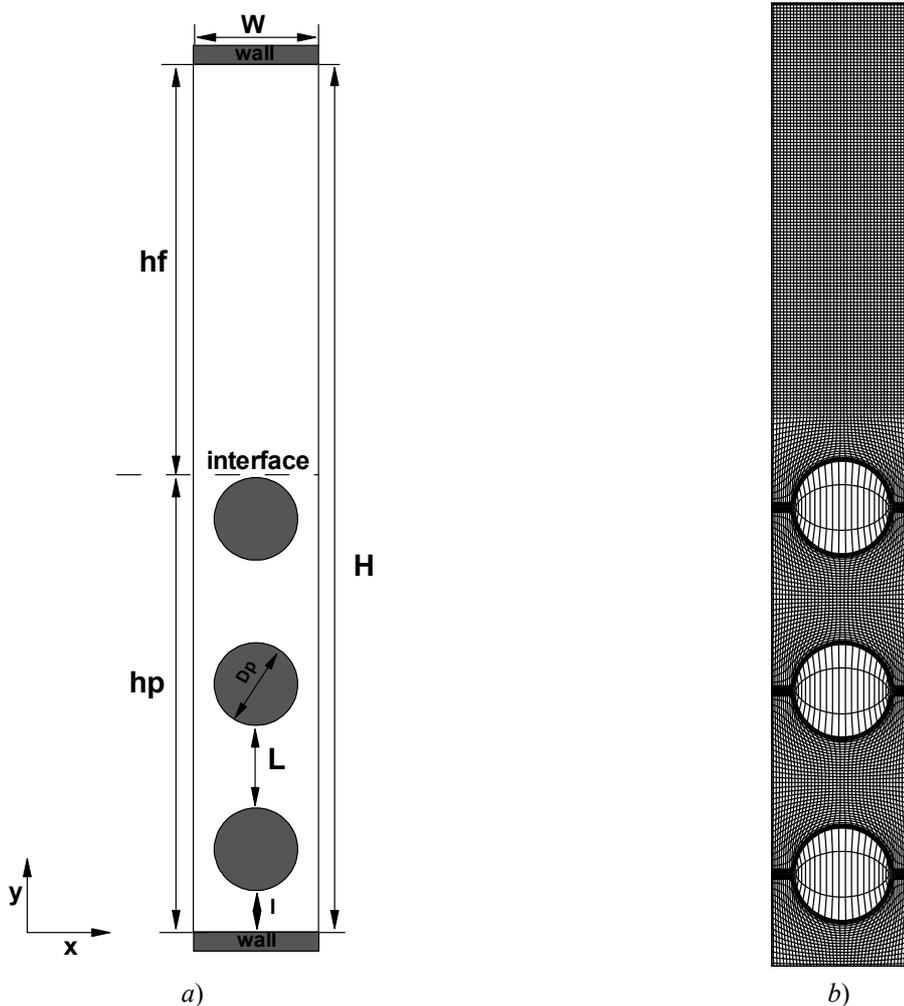
Figure 1: Geometry a), Grid computational b)
