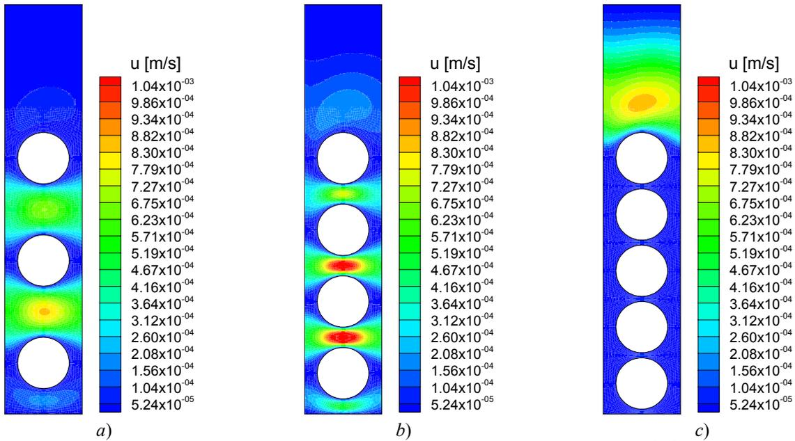
Figure 7: Velocity Field for  $Re_H=100$  e  $H=0.08\text{m}$ : a) 3 rods ( $\phi=0.7144, K=3.104 \times 10^{-6}\text{m}^2$ ), b) 4 rods ( $\phi=0.62, K=1.146 \times 10^{-6}\text{m}^2$ ), c) 5 rods ( $\phi=0.524, K=4.409 \times 10^{-7}\text{m}^2$ ).
