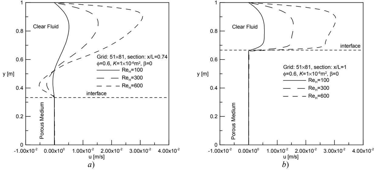
Figure 4: Effect of  $Re_H$  on velocity profiles for  $n=2$ ,  $a=1/3$ : a)  $x/L=0.74$  (valley), b)  $x/L=1$  (peak).
