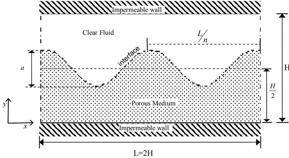
Figure 1: Channel with porous layer of wavy interface.
