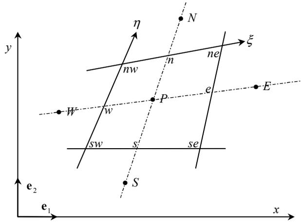
Figure 2: Notation for control volume discretization.
