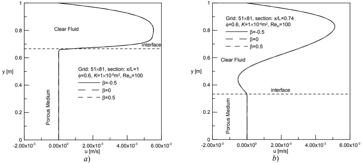
Figure 7: Effect of parameter  $\beta$  on velocity profiles for  $n=2$ ,  $a=1/3$ : a)  $x/L=0.74$  (valley), b)  $x/L=1$  (peak).
