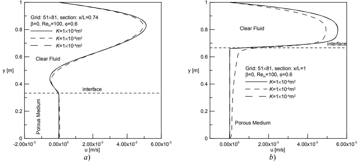
Figure 6: Effect of permeability  $K$  on velocity profiles for  $n=2$ ,  $a=1/3$ : a)  $x/L=0.74$  (valley), b)  $x/L=1$  (peak).
