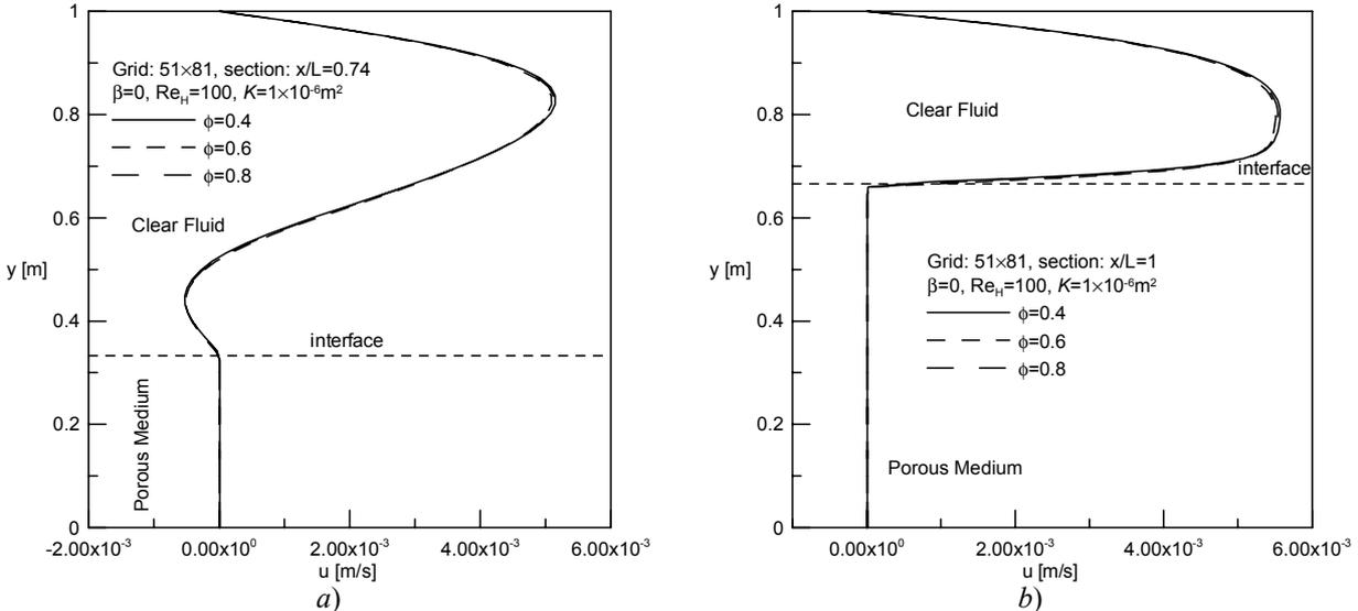
Figure 5: Effect of porosity  $\phi$  on velocity profiles for  $n=2$ ,  $a=1/3$ : a)  $x/L=0.74$  (valley), b)  $x/L=1$  (peak).
