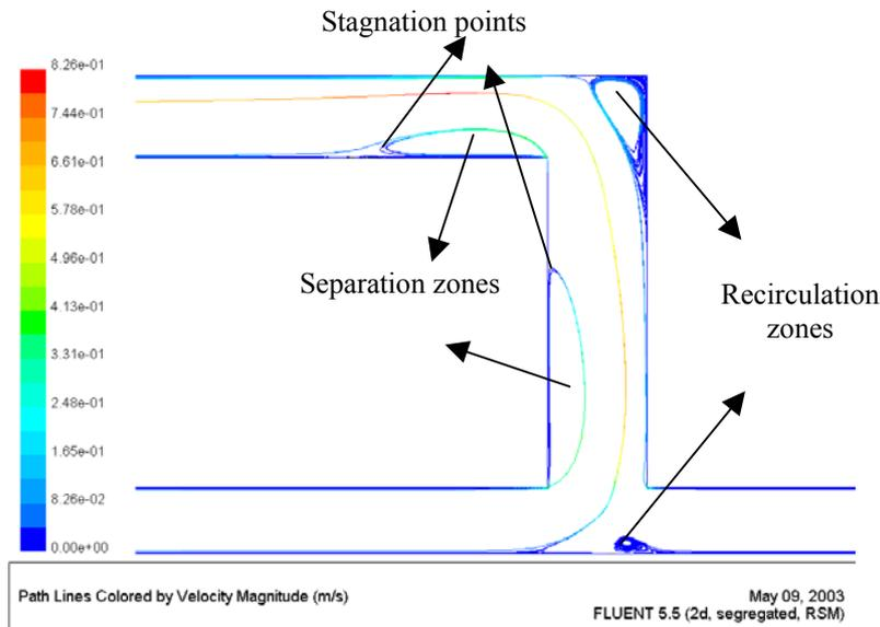
Figure 4. FAV graft flow simulation using Fluent code
