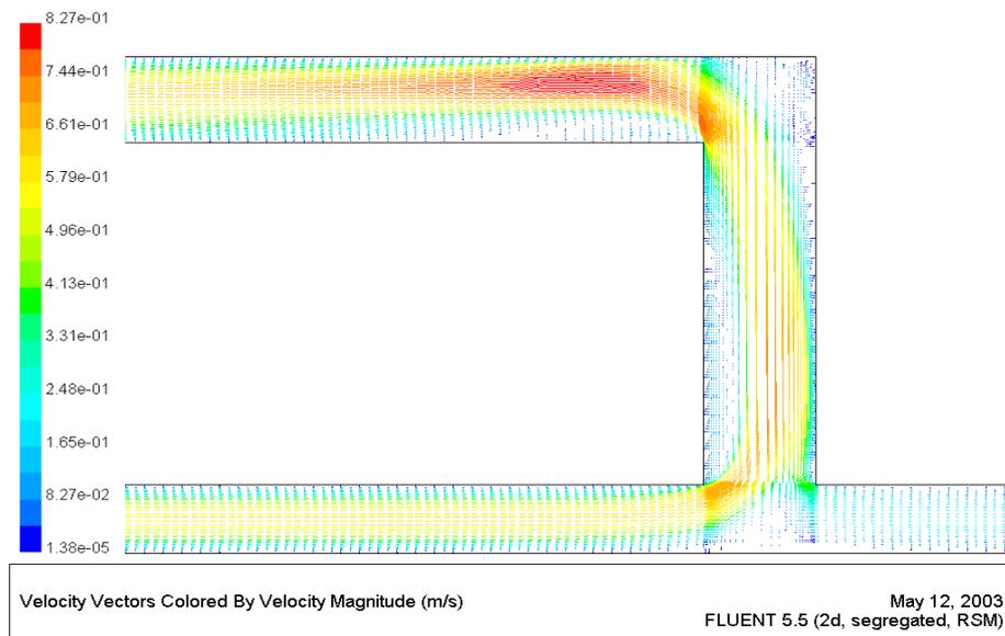
Figure 5. FAV graft flow simulation using Fluent code (flow through cranial vein).
