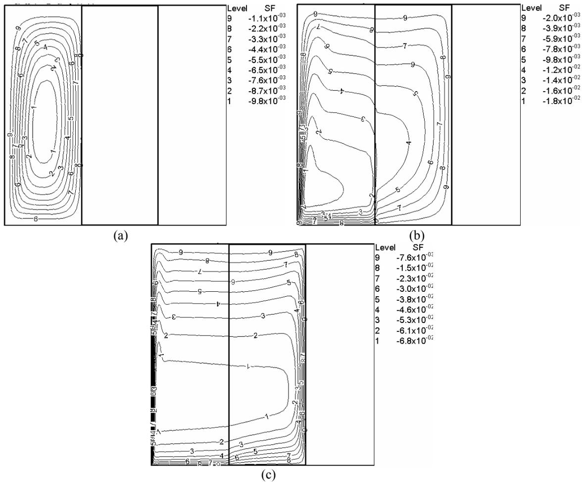
Figure 3 - Turbulent streamlines of a composite square cavity for  $Ra=10^6$ ,  $10^8$  and  $10^{10}$  with  $\phi=0.95$  and  $D_p=1$  mm.
