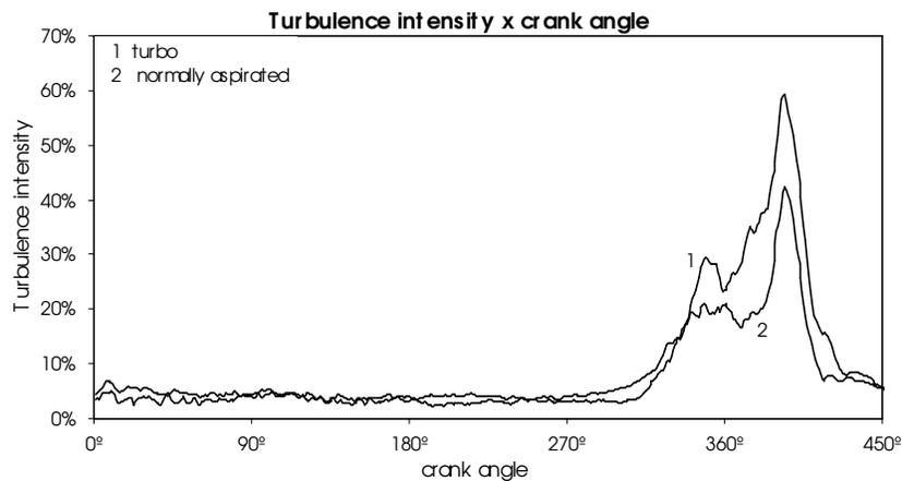
Figure 10. turbulence intensity curves.
