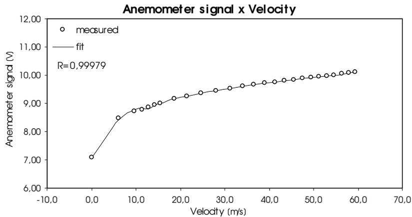
Figure 7. Constant temperature anemometer calibration curve.
