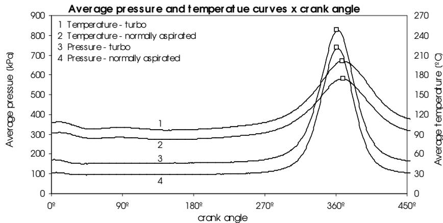
Figure 9. Ensemble average pressure and temperature curves.
