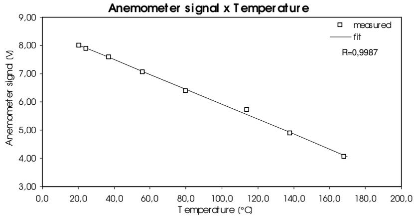
Figure 4. Constant current anemometer calibration curve.
