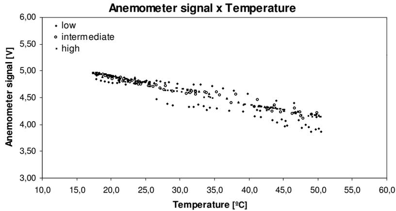
Figure 3. Constant current anemometer current adjustment calibration curves at low, intermediate and high flow velocities.
