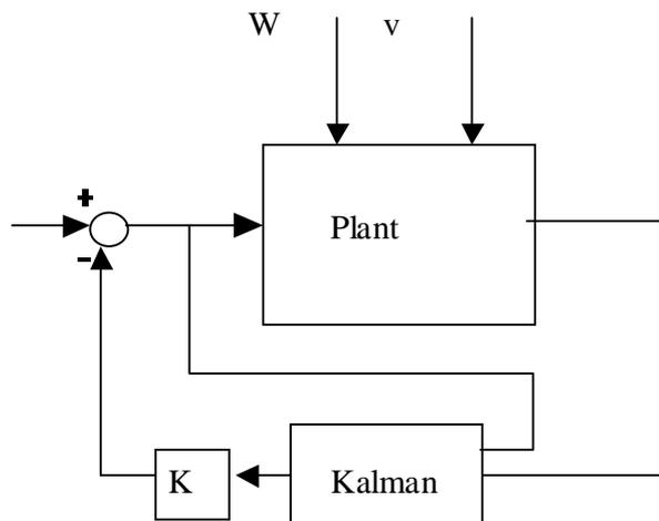
Figure 3. LQR Control Scheme with optimum state observer
