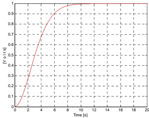
Figure 4. Angular position for a step reference
