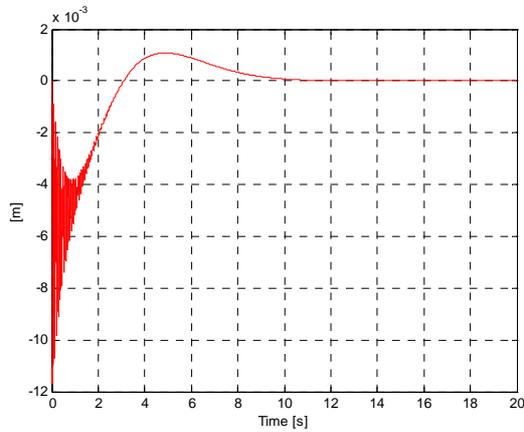
Figure 6. Transversal deformation for a step reference
