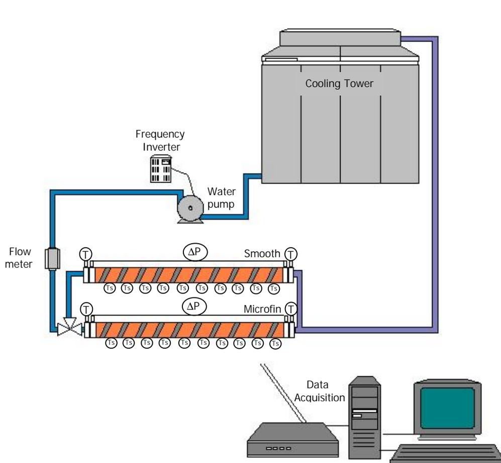
Figure 3. Schematic diagram of test facility.
