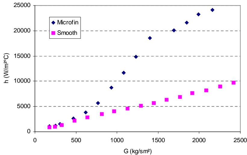
Figure 5. Heat transfer coefficients results of micro-finned and smooth tubes.
