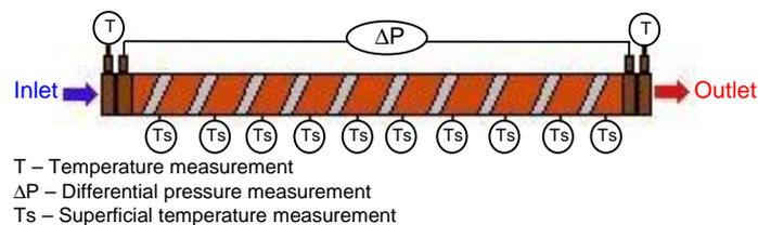
Figure 1. Diagram of tube with temperature and pressure measurements points.
