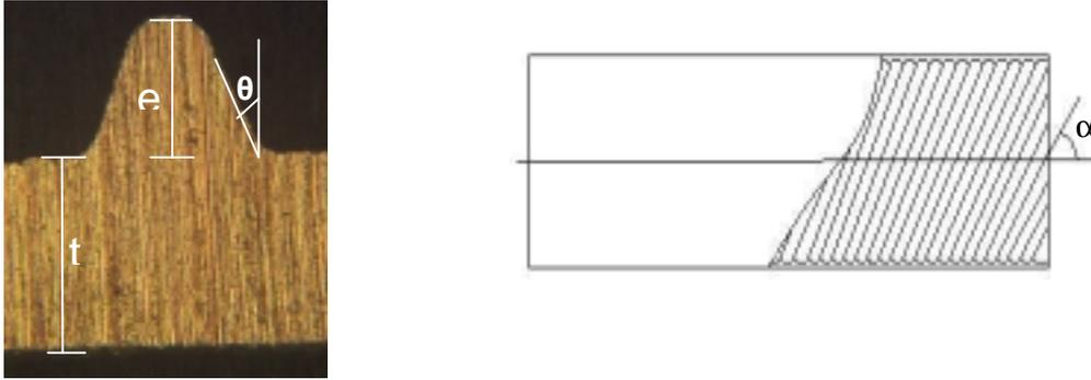
Figure 4. Micro-fin and the characteristics parameters.
