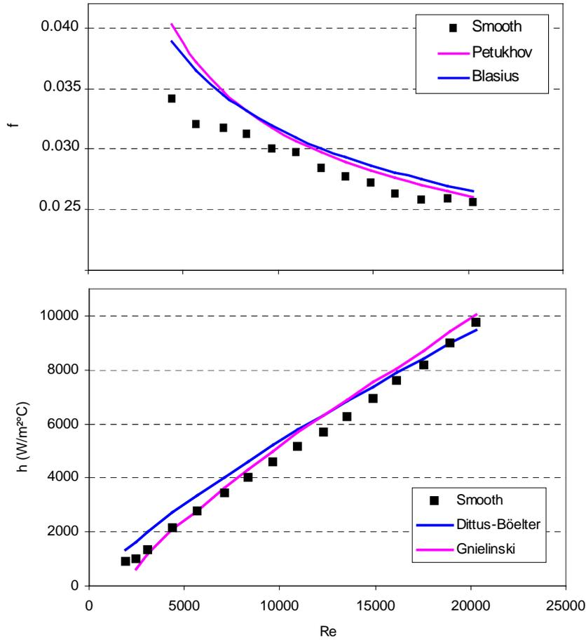
Figure 7. Friction factor and heat transfer coefficients measured and predicted for smooth tubes.
