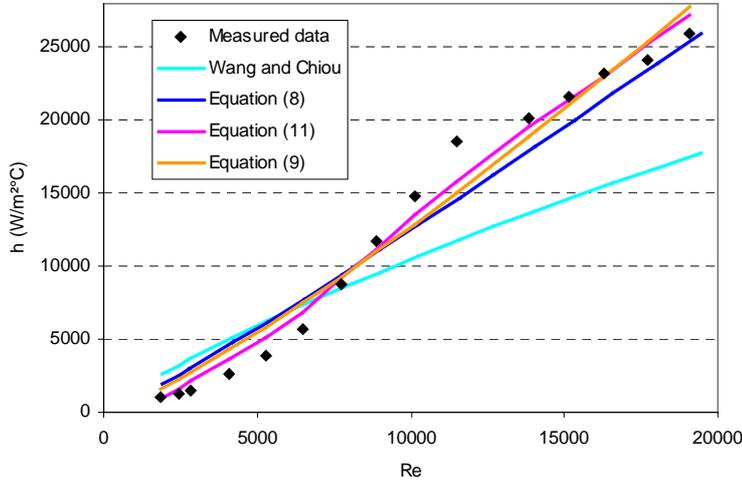
Figure 8. Heat transfer coefficient versus Reynolds number: experimental and predicted data.
