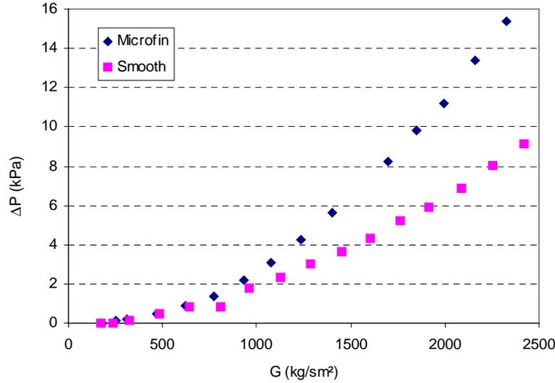
Figure 6. Experimental hydraulic behaviour of micro-fin and smooth tubes.
