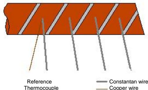
Figure 2. Thermocouples assembly for the differential wall temperature measurements.
