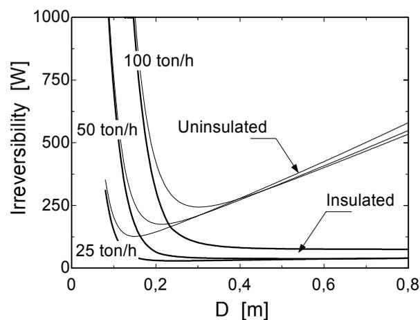
Figure 3. Irreversibility rate vs. internal diameter for different steam flow rates (Scenario 1)
