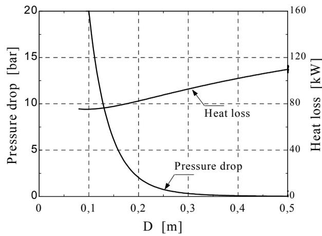
Figure 5. Trade-off between heat loss and pressure drop for 25 ton/h vs. internal diameter of the pipeline (Scenario 2).
