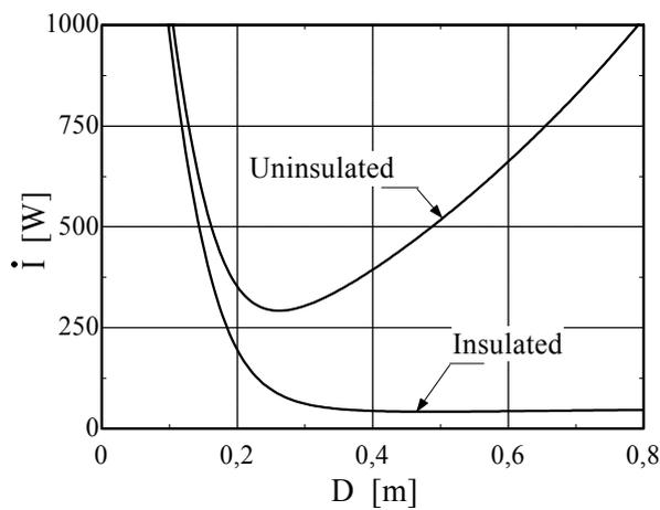
Figure 6. Irreversibility rate vs. internal diameter, for uninsulated and insulated pipeline (Scenario 2)
