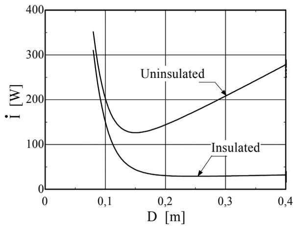
Figure 4. Irreversibility rate vs. internal diameter (uninsulated and insulated pipelines, Scenario 1: 45 bar; 400°C; 100m; 25 ton/h)
