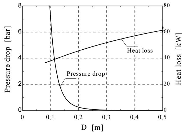
Figure 2. Trade-off between heat loss and pressure drop for 25 ton/h vs. internal diameter of the pipeline (Scenario 1).
