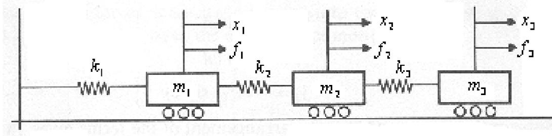
Figure 2 – System, mass –spring, equivalent of the beam with three degrees of freedom.
