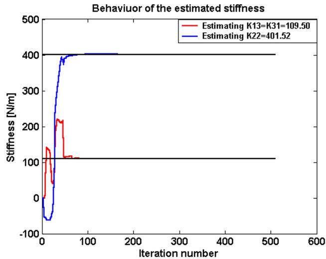
Figure 7. Behavior of stiffness estimation  $K_{13}$ ,  $K_{31}$ ,  $K_{22}$
