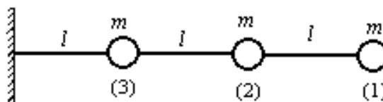
Figure 1 – Representation of the cantilever beam, with concentrated masses.
