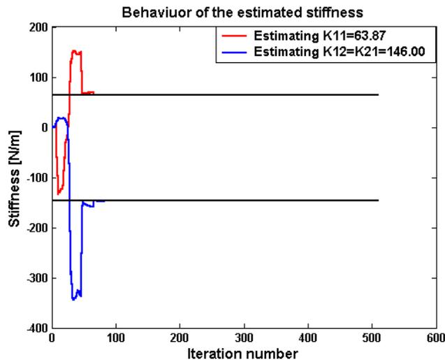
Figure 6. Behavior of stiffness estimation  $K_{11}$ ,  $K_{12}$ ,  $K_{21}$
