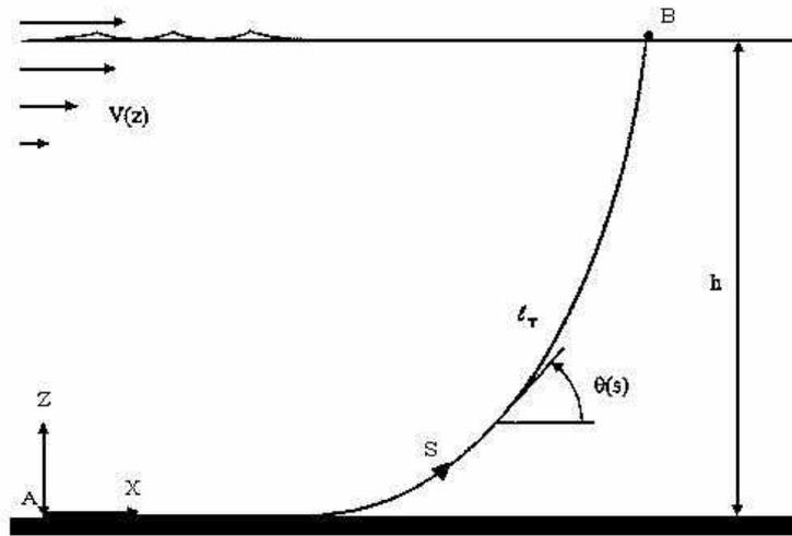
Figure 1. Two-dimensional static configuration and geometric definitions (adapted from Aranha et al, 1997)
