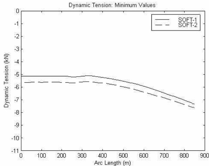
Figure 3. Minimum dynamic tension forces comparison
