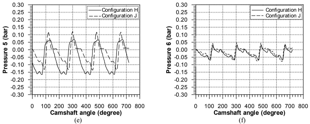
Figure 6- Pressure signals from the pressure transducers P1 (a), P2 (b), P3 (c), P4 (d), P5 (e) and P6 (f) at 2000 rpm camshaft speed.
