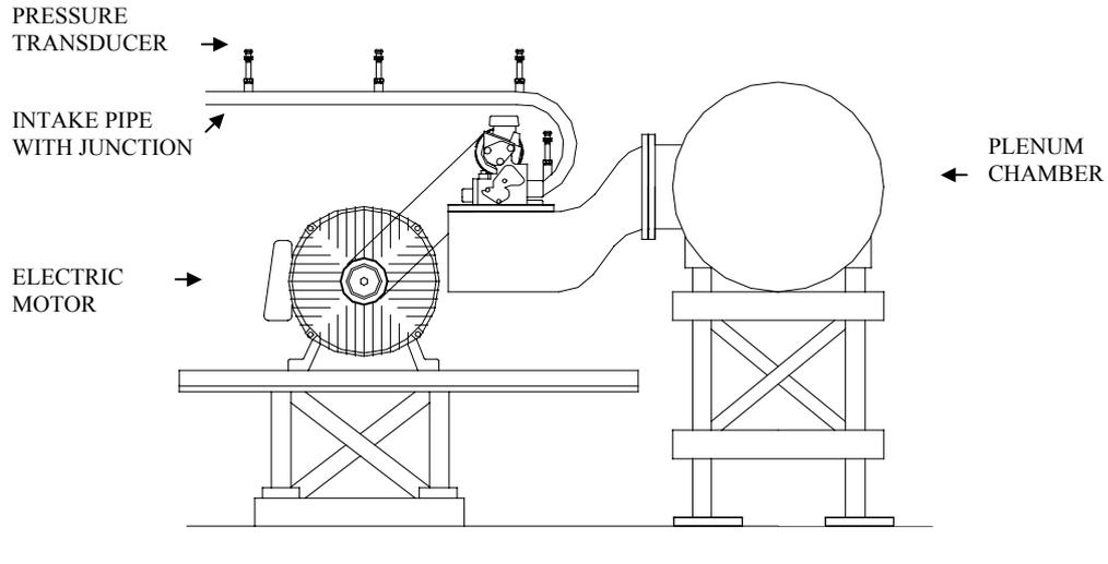
Figure 3 - Schematic drawing of the experimental rig.
